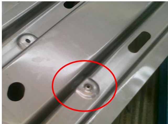
Figure 128: Actual reinforcement channel with fixation points from seat belt guides.
