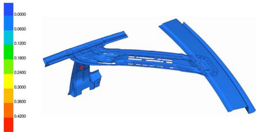
Figure 136: Graphic representation from Detail A on Figure 135, regarding displacement [mm]. ( Volkswagen Simulation Department )
