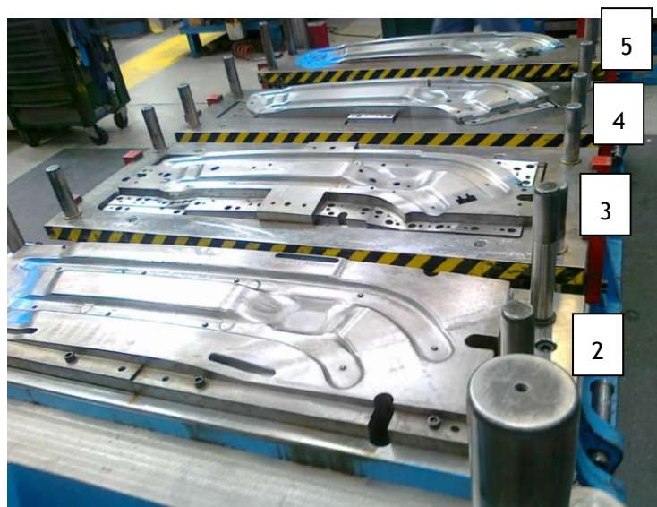
Figure 36: Actual part press tool with 4 different operations. ( Gestamp Portugal )
