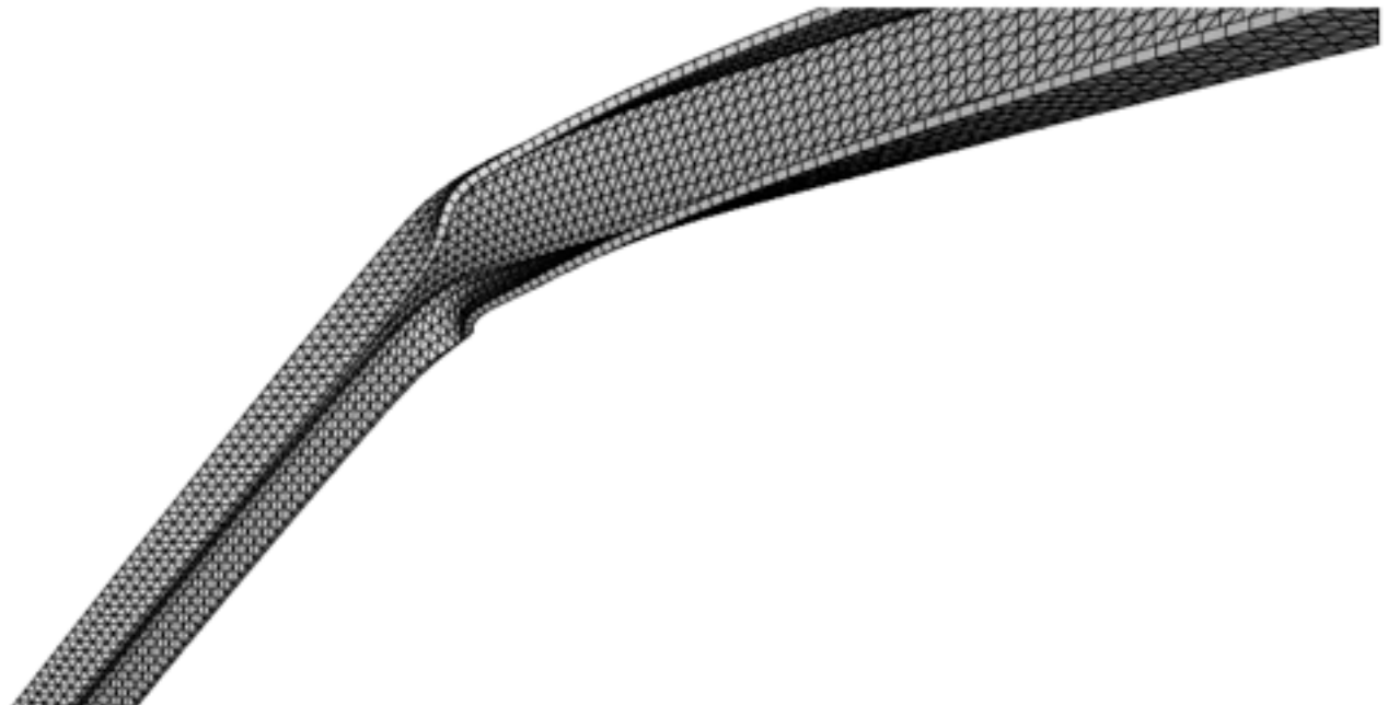
Numerically obtained elasto-plastic flange buckling (thickness extrusion was performed)
