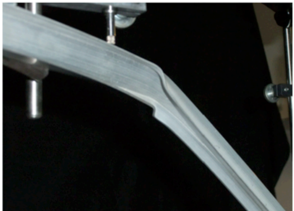
Experimentally observed elasto-plastic flange buckling
