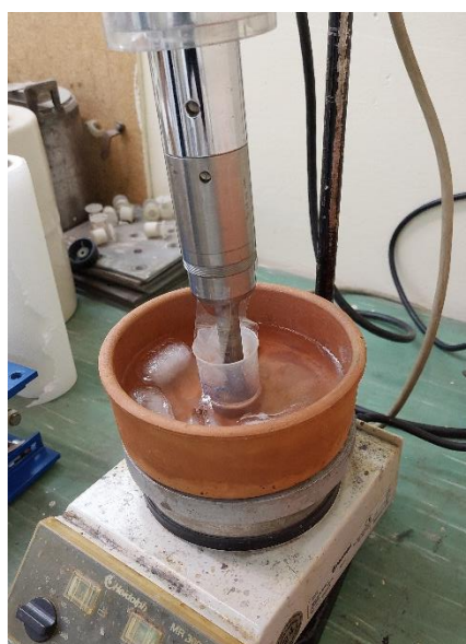
Image 30: Ice bath and sonication on the sample for mixing
