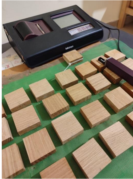
Image 24: Equipment on top of the sample measuring the roughness
