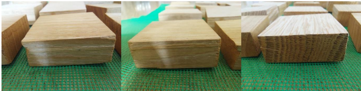
Image 65: Some of the visible defects after weathering for 3 months
