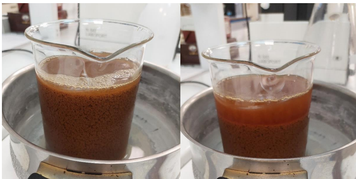
Image 15: Solution with the lignin going through decantation after the addition of water on the mixture
