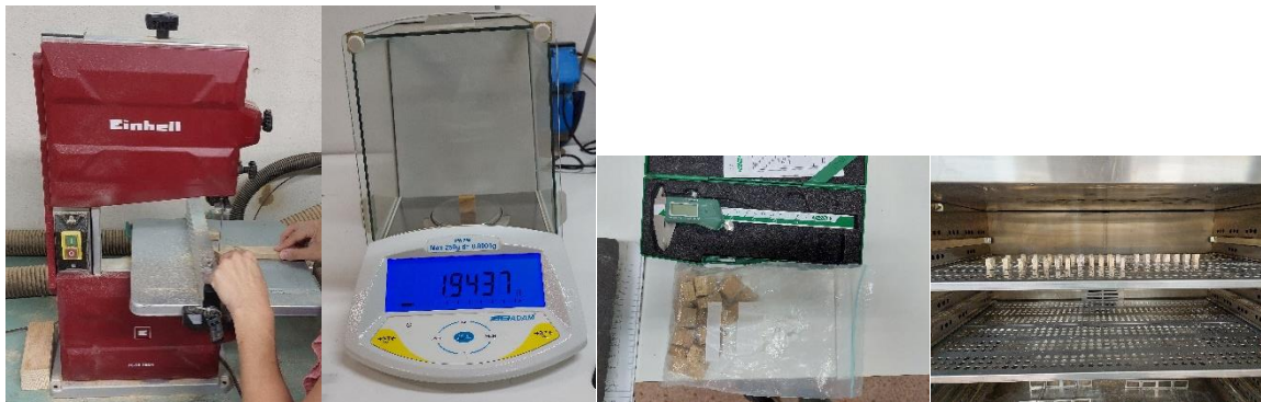
Image 25: Cutting, measuring, and drying the samples
