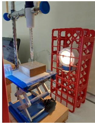
Image 18: System created to photograph the drops for contact angle.
