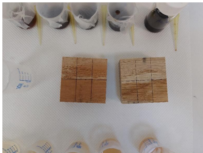
Image 44: Substrates during cure process after the application of coatings with acetone and nanolignin
