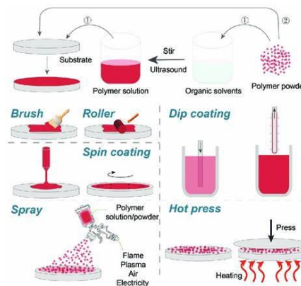
Image 13: Some application methods for coatings (source: A review on tribology of polymer composite coatings - Scientific Figure on ResearchGate. Available from: https://www.researchgate.net/figure/Schematic-diagram-of-various-methods-for-preparing-polymer-coatings_fig3_347224053 [accessed 22 Sept 2024])
