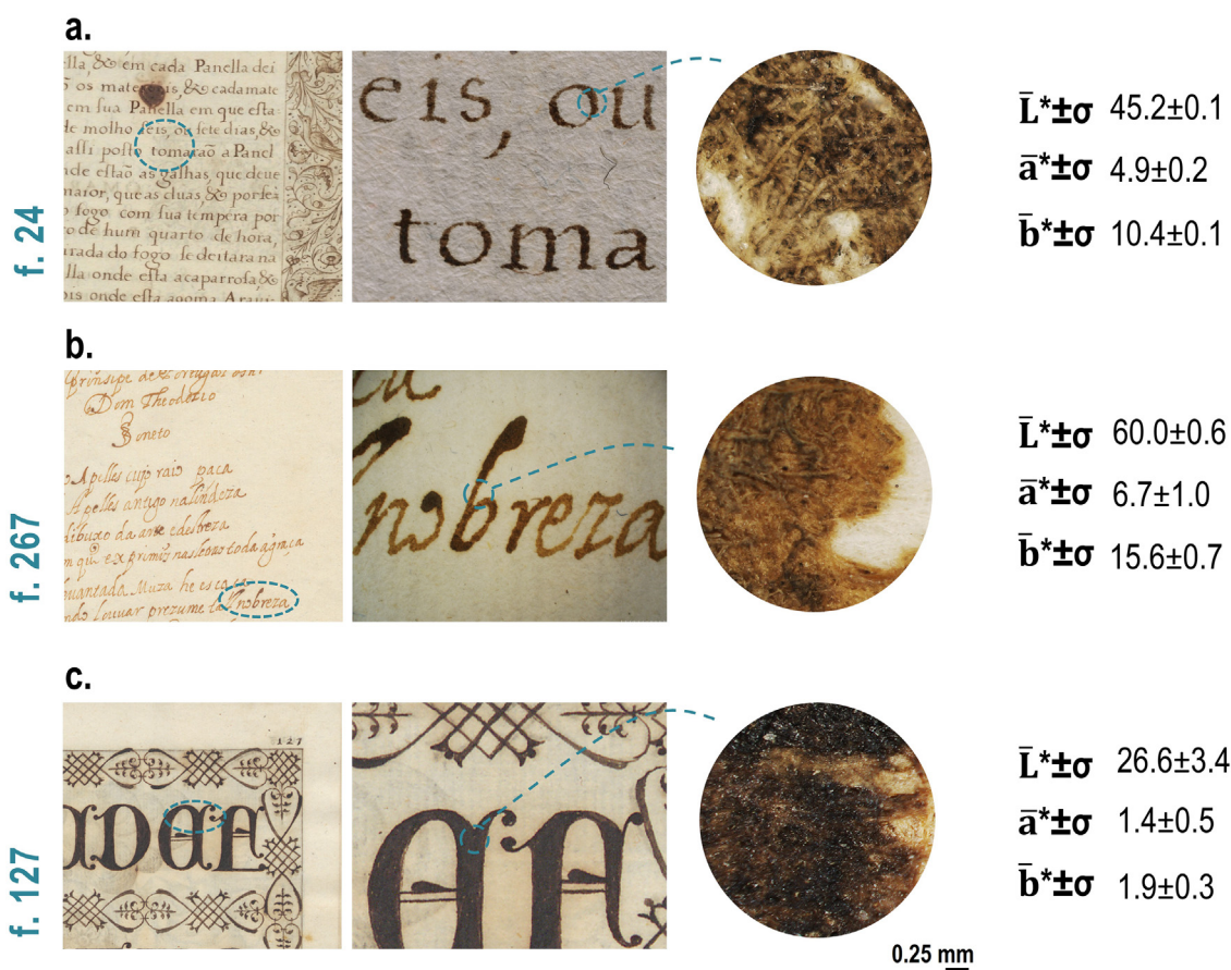
Fig. 1. Photographic details, 3D digital microscopic images illustrating morphological aspects of representative inked areas and corresponding average L^*a^*b^* values and std ( \sigma ) values. Text block with a) rusty-brown hue (f. 24); and b) golden brown hue (f. 267); c) calligraphic writing with a dark black shade (f. 127).
