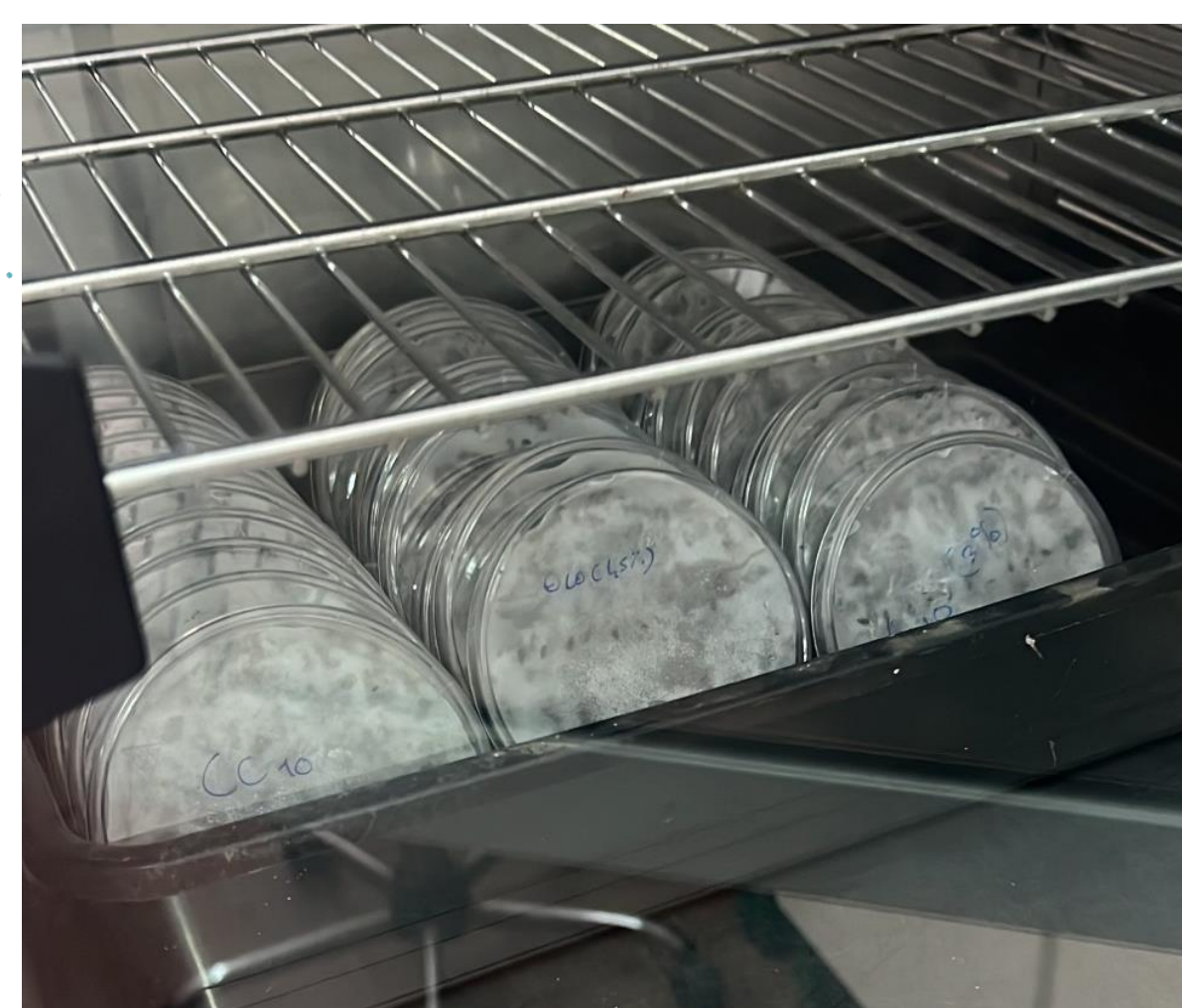
Petri dishes with Lactuca sativa L. seeds on soil with different biochar concentrations in the incubator
