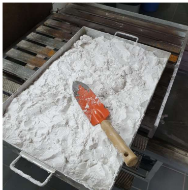
Dry, Disintegrated Carbonate Sludge
