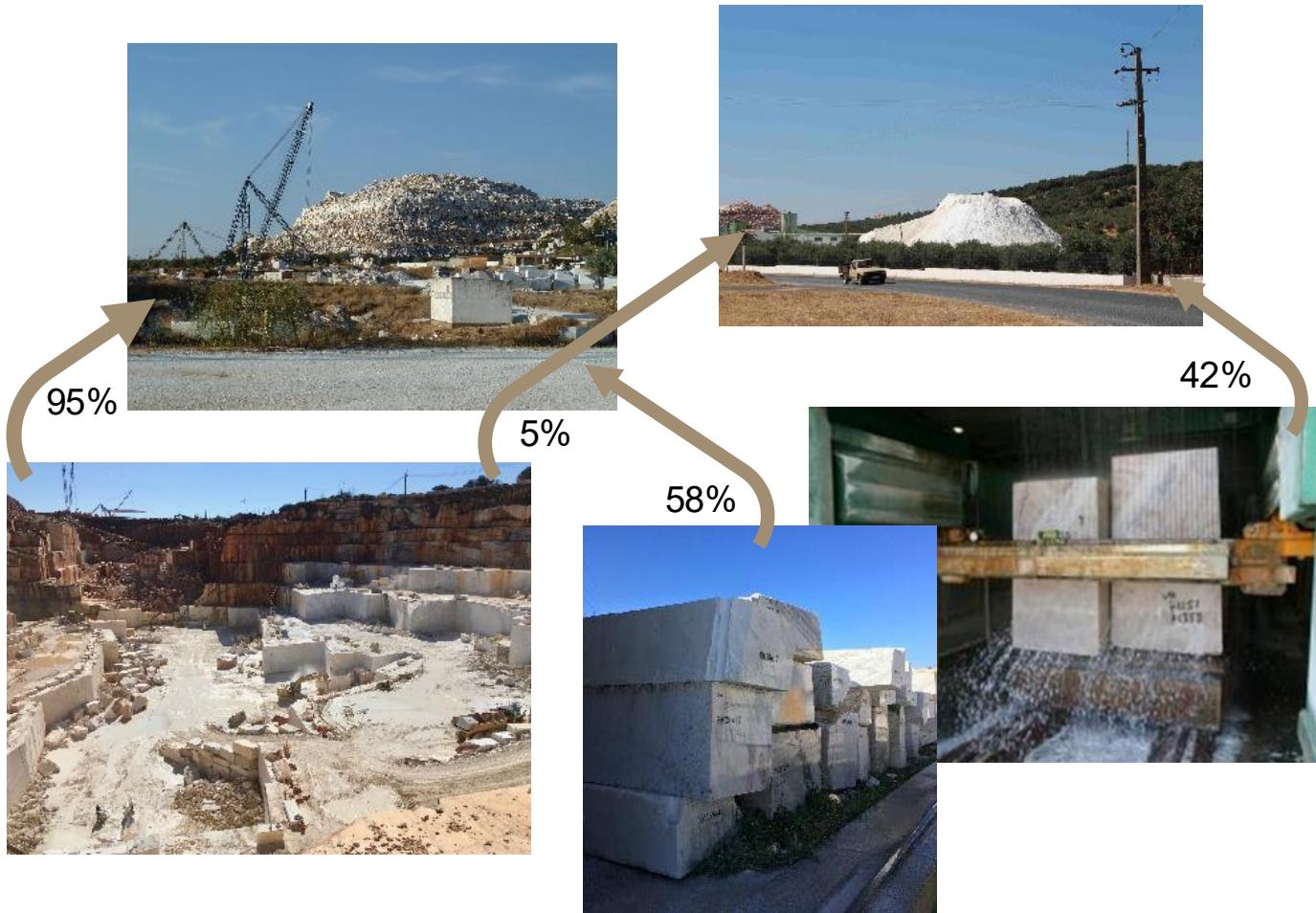
The carbonate dimension stone extractive and processing industry produces large amounts of wastes later deposited in heaps and deposits of carbonate sludge.
