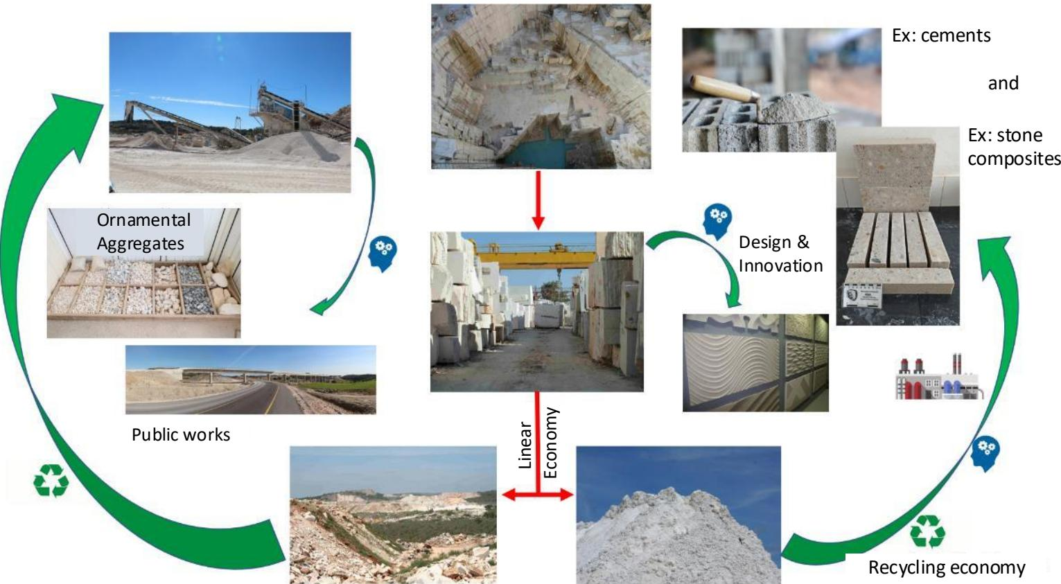
Creation of new products using waste from the extraction and processing of carbonate ornamental stone.
