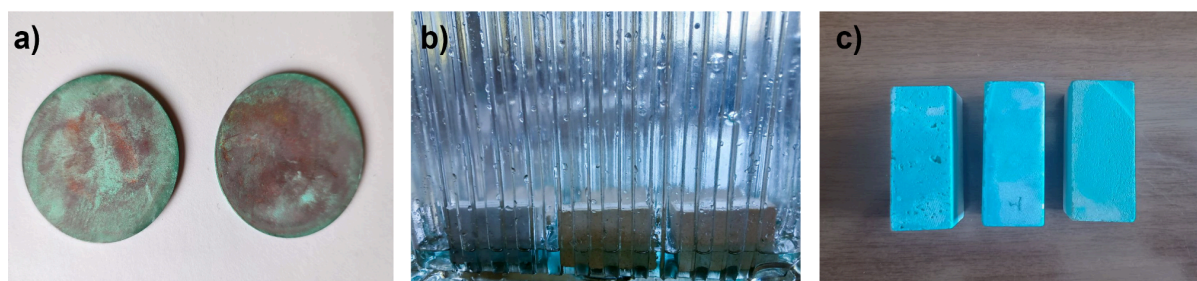
Figure 11. Photos of a) bronze disks after sulfate-induced corrosion, b) experimental setup for the immersion of stone blocks, and c) stone blocks after leaching of bronze corrosion products.
