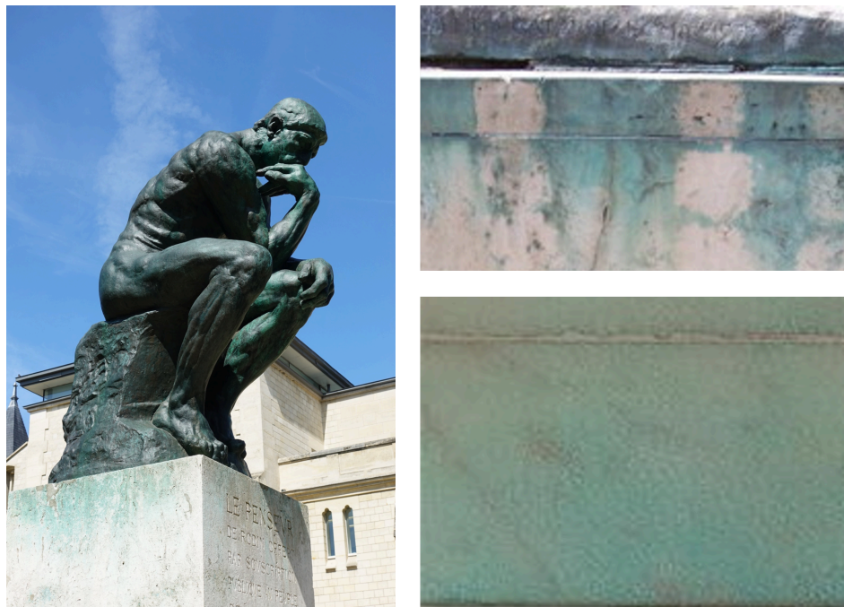
Figure 5. Digital images of copper staining on stone including The Thinker by Rodin, Student Statue in the Sapienza University of Rome, and a stone piece in the Museum of Modern Art in Aalborg, Denmark. 13,45,51
