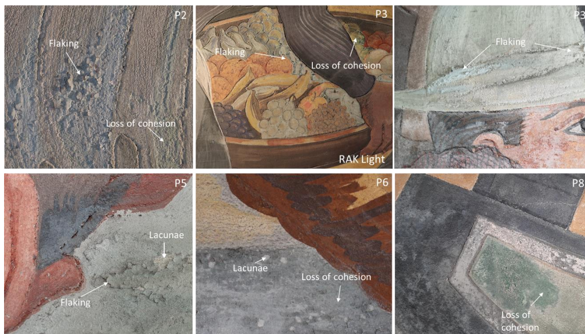
Figure 5. Photographic documentation in visible and visible ranking light of deteriorated paint layers.
