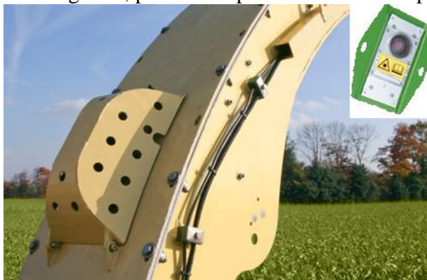
Krone crop moisture sensing system
