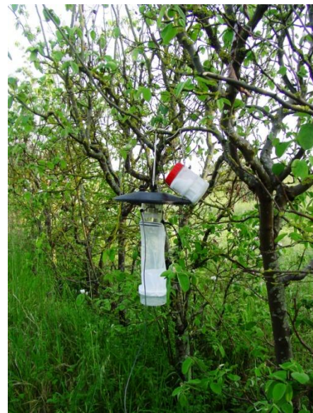
Figure 16. CDC light trap baited with CO 2 .
