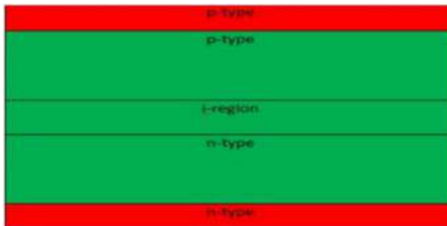
Fig 1: standard structure of p-i-n solar cell.
