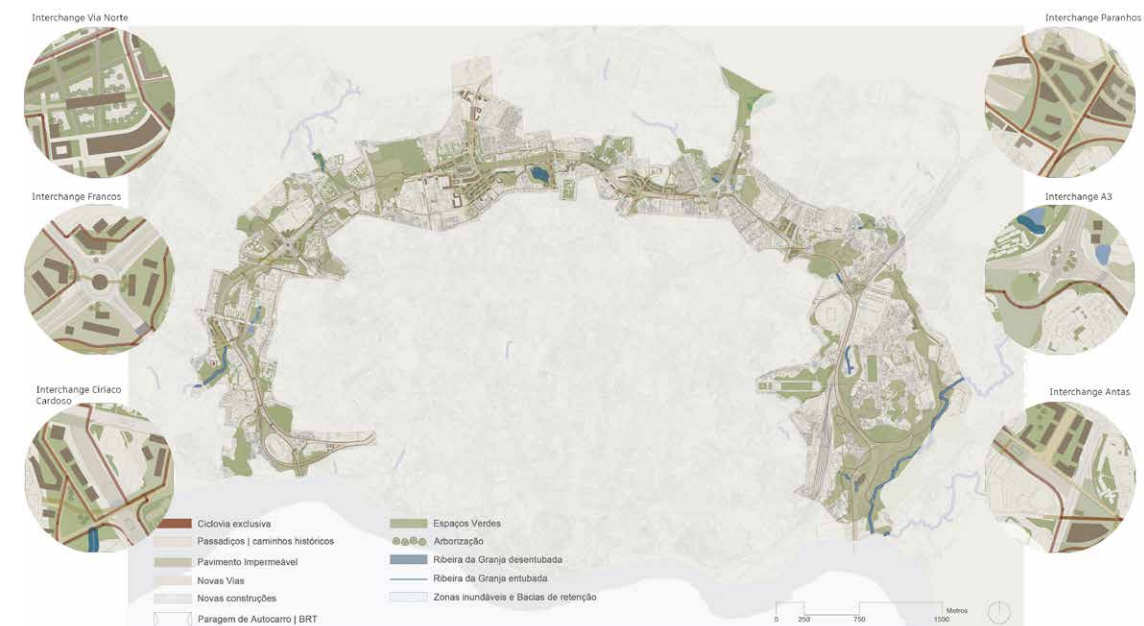
Figure 6. The proposal and the transformed interchanges. The resolution of the interchanges of Ciriaco Cardoso, Paranhos and Antas was based on the reconstruction of the pre-existing connections between the two banks of the VCI.
