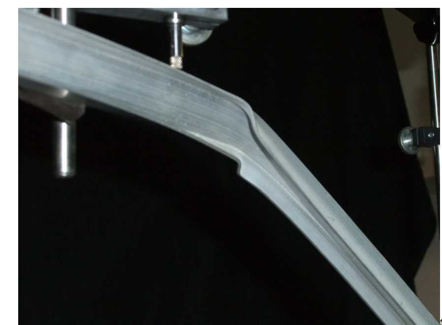
Experimentally observed elasto-plastic flange buckling
