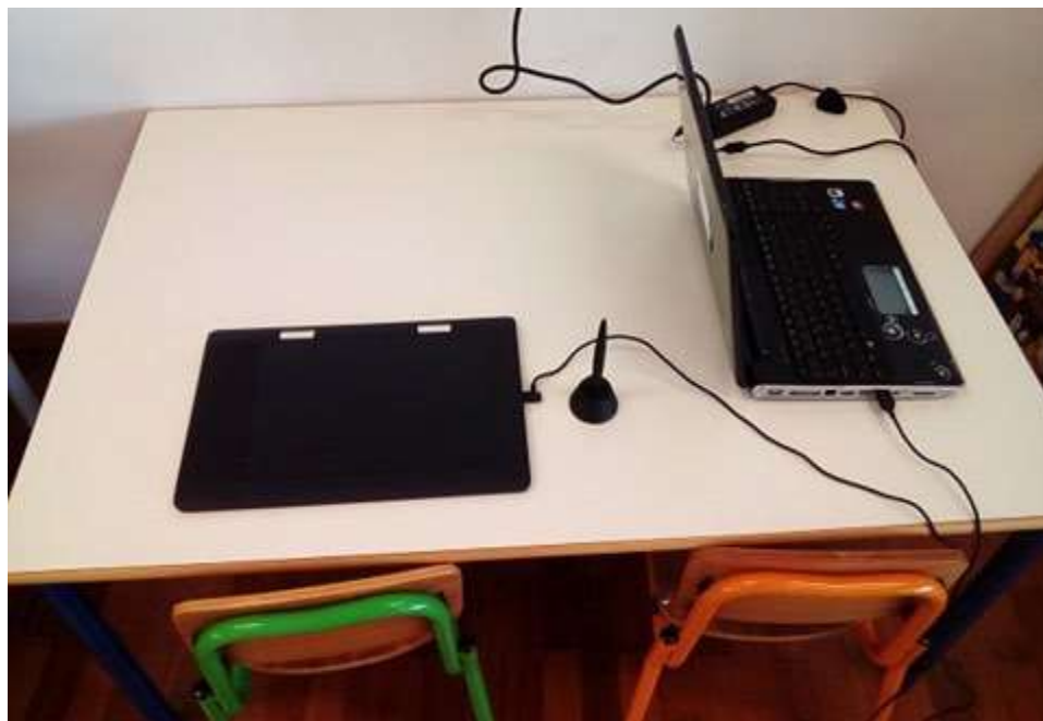
Figure 1. The experimental graphomotor setup with a pen tablet, school desk, and chairs. The experimenter was seated on the right side and could monitor the pen movements in real time on a laptop.
