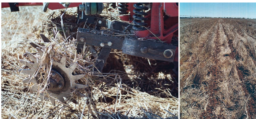
Figure 9 Row-cleaners used for crop establishment into residue-rich no-till seedbed.
