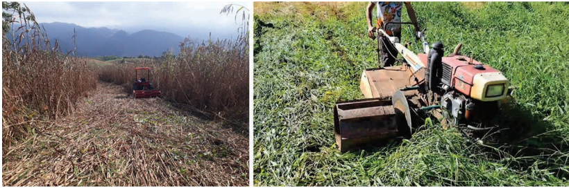
Figure 10 Roller crimper to terminate the cover crop consisting of pearl millet (left); two-wheel walking tractor, equipped with a roller, cutting disk and straight rotary device as row opener (right).
