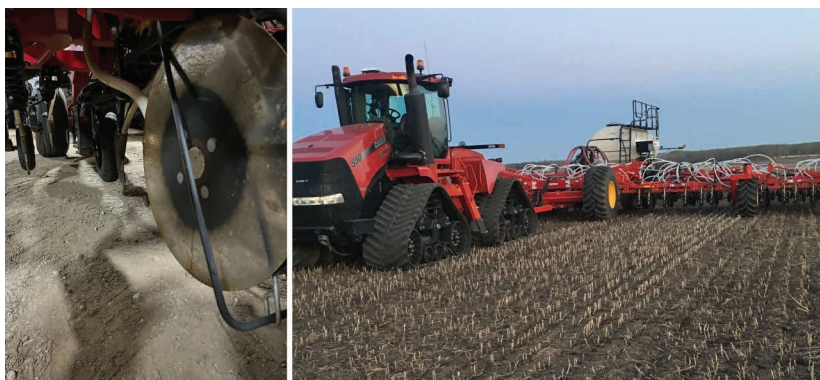
Figure 35 Planting equipment used on the farm with knife opener for seed placement and discs for fertilizer banding.
