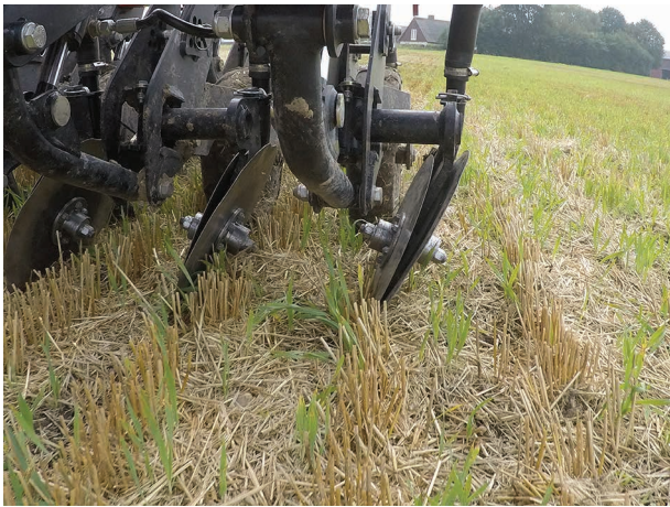
Figure 6 No-till with strongly inclined disc openers for minimum soil disturbance.
