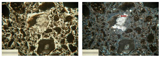
Figure 17: Calcite crystal within the sediment. Left: PPL; right: XPL. Bar length: 1 mm.
