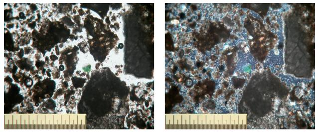
Figure 18: Green particle in the foundation deposit sediment, representing malachite or copper corrosion product. Left: PPL, right: XPL. Bar length: 1 mm.
