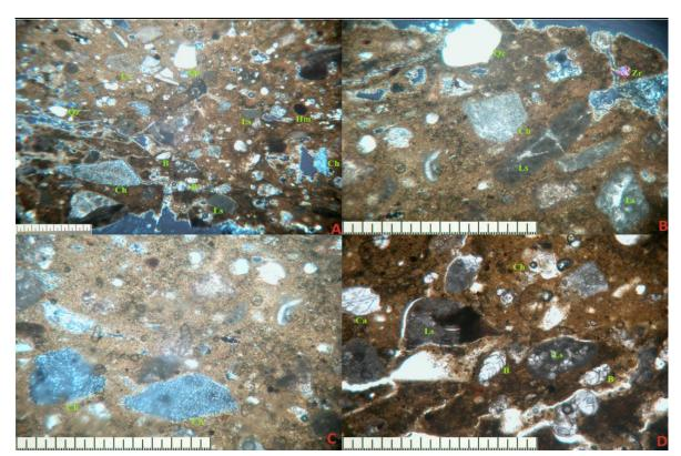
Figure 19: photomicrographs of the cornet sample under the petrographic microscope. Scale bar: 1 mm. Legend: A) Qzquartz, Ls- limestone, Ch-chert, Hm-hematite, B- Bolivina sp. Microfossil (XPL). B) Ch- chert (XPL). C) Qz-quartz, Zrzircon, Ch- chert, Ls-limestone (XPL). D) B- Bolivina sp.Ch- chert Ls- limestone Ca-calcite (PPL)
