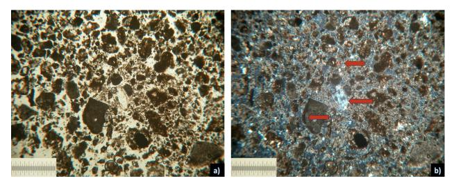
Figure 16: Photomicrographs of the sediment block taken from the foundation deposit, two views of the same location where the left was taken under plane-polarized light (PPL) and the right between crossed polarizers (XPL). The lower arrow shows a clay-coated grain of limestone. The middle arrow points at a gypsum spar crystal. The upper arrow shows a zircon particle within the silt fraction. The scale bar length is 1 mm.
