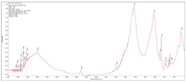
Figure 22: FTIR pattern of the sample L35 B1070( ash)
