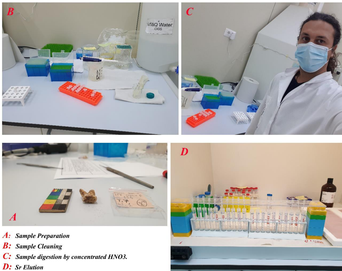
Fig.8: Different steps of sample preparation A: Enamel Extraction B: Sample Cleaning C: Sample digestion by concentrated HNO 3 D: Sr Elution.
