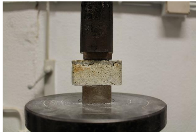
Figure 7. Compressive strength test.
