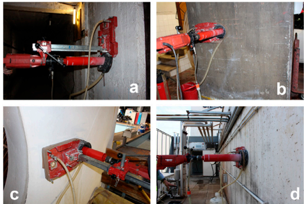
Figure 1. Images of concrete sampling campaign: (a) IRF (1938); (b) FRAN (1971); (c) JRP (1987); (d) PCV (1998).
