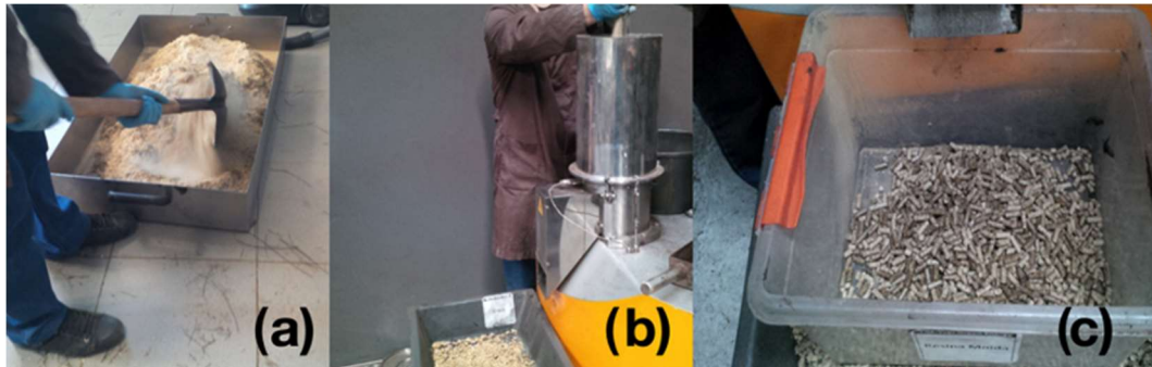
Figure 2. Pellet production process using a KAHL laboratory scale pelletizing machine with a production capacity of 25 kg/h. (a) The mixing process for homogenizing the product to be pelletized, mainly to ensure that the humidity is uniform; (b) the equipment used to produce the pellets; (c) the final result. The pellets were produced exclusively with Acacia dealbata biomass.
