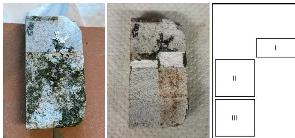
Figure 5.15. Sample tablet for ns-IR laser treatment: before cleaning (left), after cleaning (middle), and three zones with different treating parameters (right).
