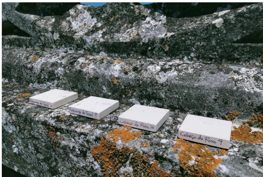
Figure 6.3. Sample tablets placed on the monastery roof (from left to right, the 1 st and 3 rd are deposited with SiO x film, the 2 nd and 4 th are uncoated).
