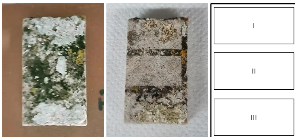
Figure 5.9. Sample tablet for ps-UV laser treatment: before cleaning (left), after cleaning (middle), and three zones with different treating parameters (right).
