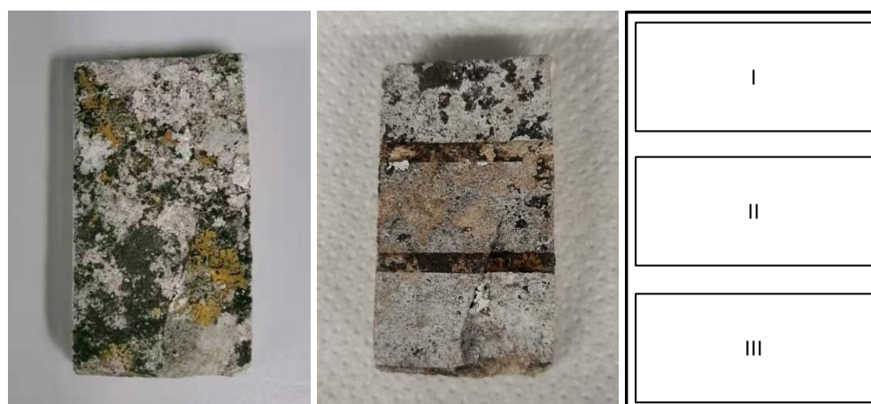
Figure 5.12. Sample tablet for ps-IR laser treatment: before cleaning (left), after cleaning (middle), and three zones with different treatment parameters (right), see also Table 5.3.
