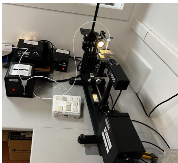
Figure 2.6 ramé-hart Model 210 Goniometer/Tensiometer during static contact angle measurement on a sample
