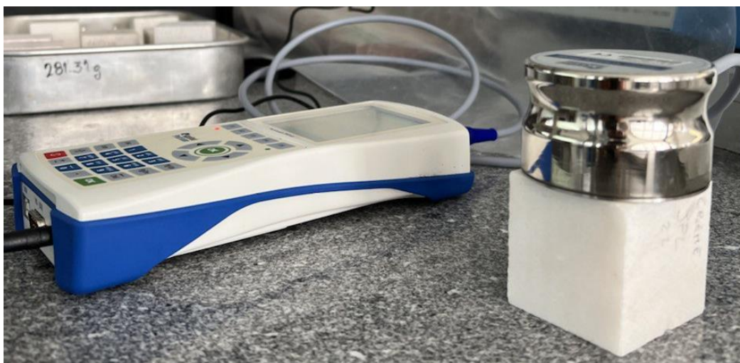
Figure 2.4. Heat Transfer Analyser ISOMET 2104 with the metal measuring probe on top of the stone sample
