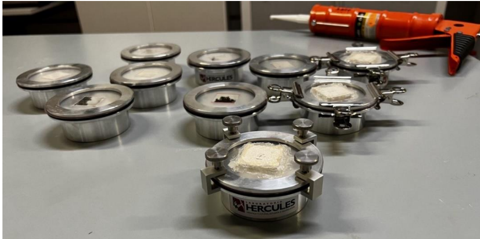
Figure 2.6. The sets of containers, wet cotton, and the specimens glued to the plastic covers.
