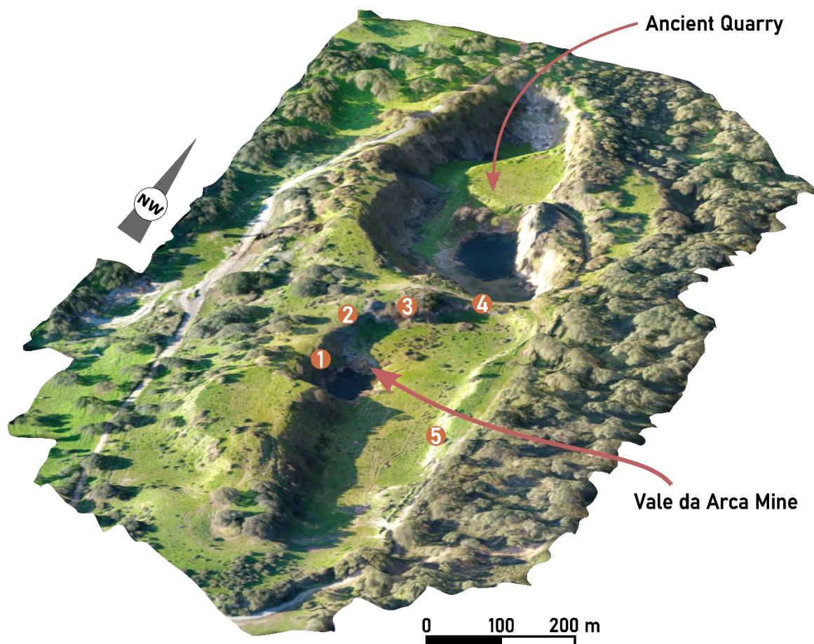
Figure 6.5. Digital elevation model with overlapped orthophotomaps of the Vale da Arca Mine area, which is the result of drone aerial imaging and latter 2.5D model construction using QGIS plugin QGIS2ThreeJS. The pinpoints on the model correspond to locations where several geodiversity features can be observed. These locations are described throughout the manuscript.
