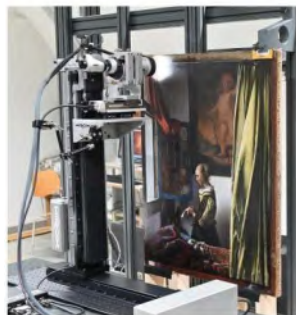
Horizontal inspection: Fully automated XYZ Gigapixel, T-stand scan system, SKD Dresden
