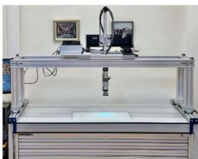
Vertical inspection: Bridge stand with Motorized XYZ for textile inspection, Hirayama Studio, British Museum
