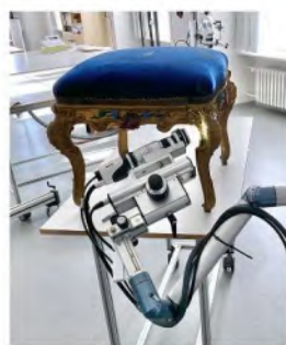
New flexible arm stand with auto Z for inspection of 3D objects in 3D
