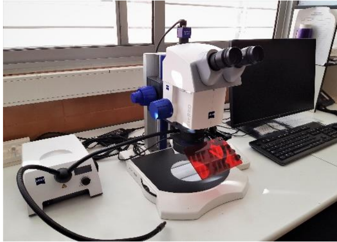
Figure 2.7: Photograph of the ZEISS SteREO Discovery.V8 optical microscope used in the surface morphological observation of the glasses.
