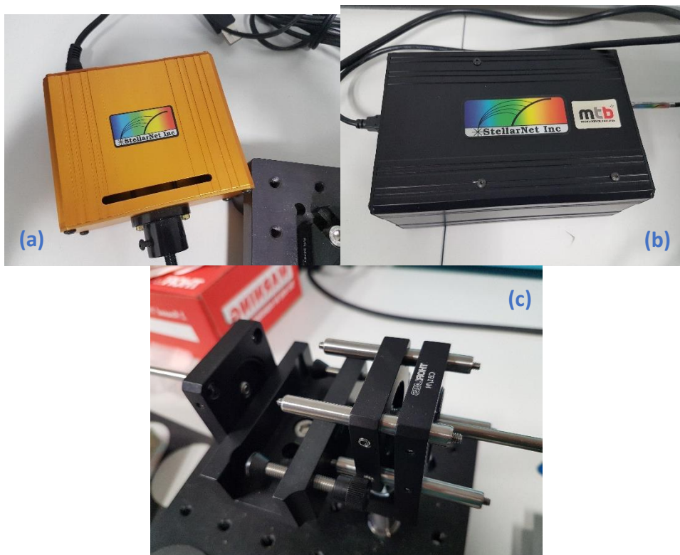
Figure 2.6: Images of the different components of the spectrometer: (a) SL1-CAL light source, (b) StellarNet unit and (c) sample holder
