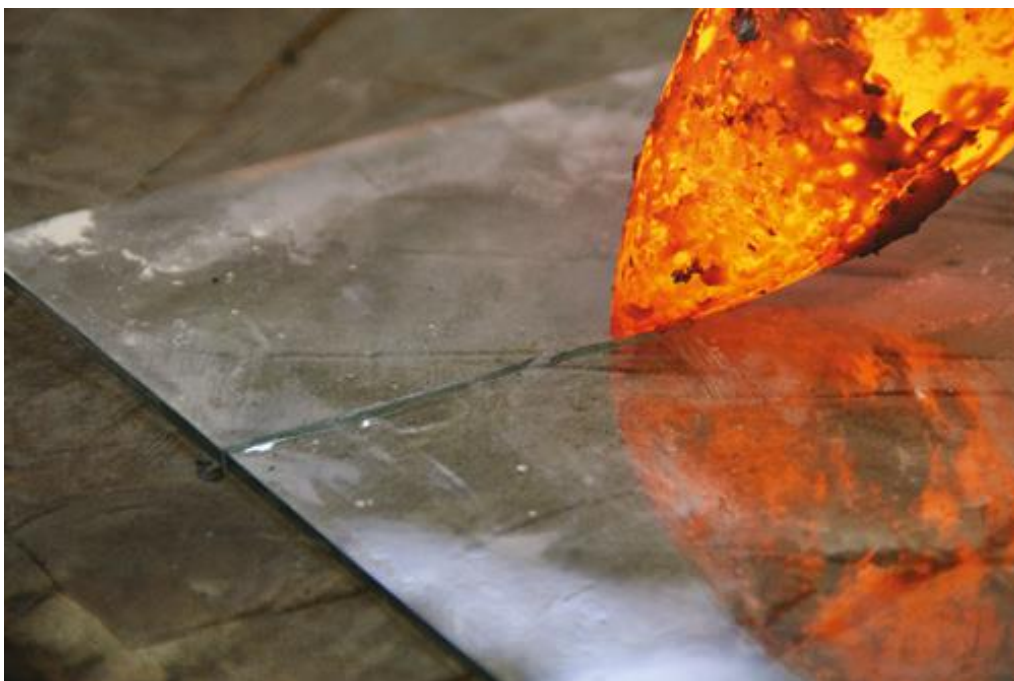
Figure 1.10: A heated dividing iron causing a crack to form on a glass sheet. (Image from [Carson Pastan2019])
