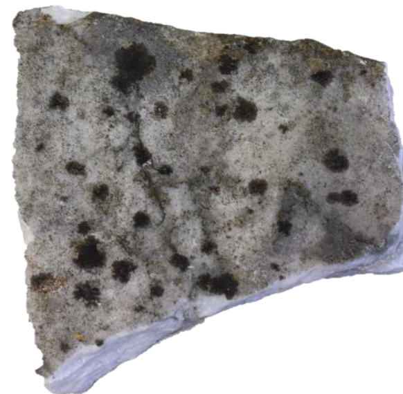
Material: Marble Code: White Estremoz Marble Provenance locality: Estremoz Problems: Slab surface oblique to foliation. OBJECTIVE: Remove bio-colonization and clean the surface stains without altering the surface.
