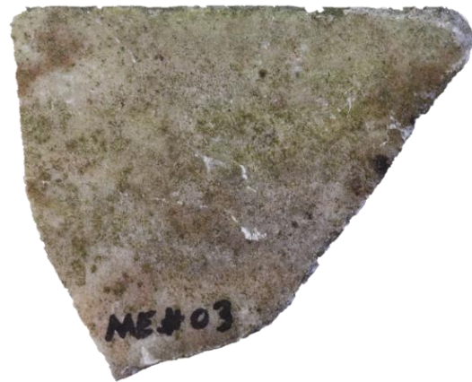
White Estremoz Marble with pink veins, slab surface oblique to foliation. Provenance locality: Vila Viçosa, Lagoa
