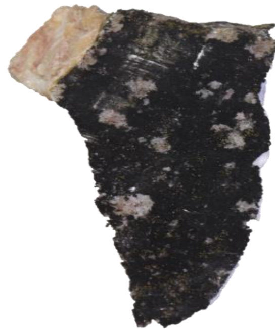
Material: Marble Code: Cream Estremoz Marble Provenance locality: Vila Viçosa, Lagoa Problems: Slab surface oblique to foliation. OBJECTIVE: Remove bio-colonization and clean the surface stains without altering the surface.
