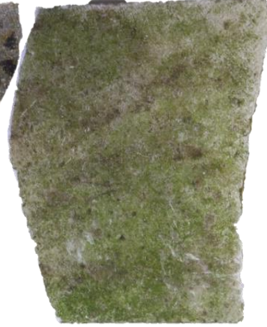
White Estremoz Marble with pink veins, slab surface oblique to foliation. Provenance locality: Vila Viçosa, Lagoa
