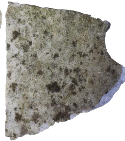
White Estremoz Marble with well-defined foliation parallel to the slab surface. Provenance locality: Estremoz
