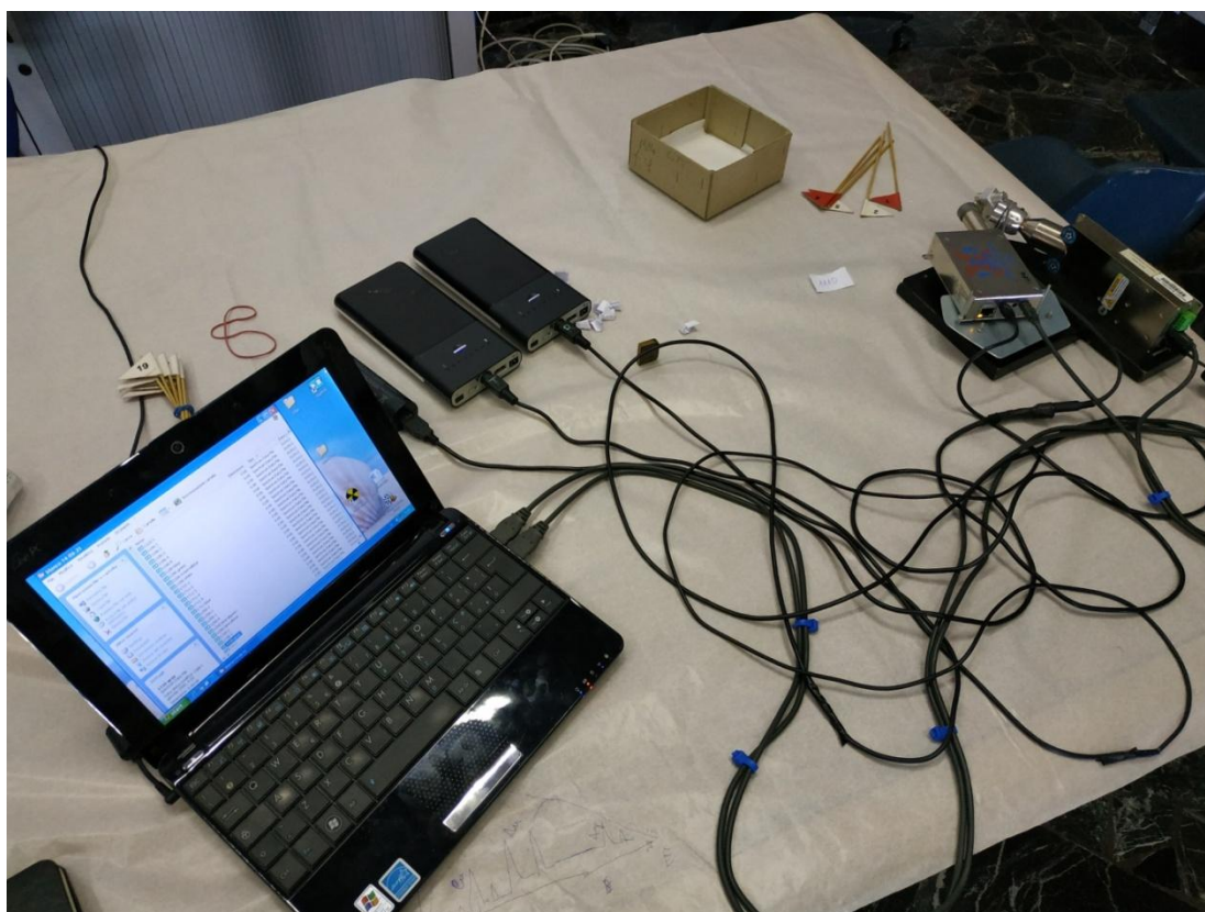
Photography 5. XRF equipment and setup used for the analysis.
