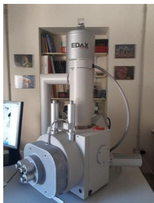
Figure 4.2 Scanning Electron Microscope FEI-QUANTA 400 (SEM-EDAX)
