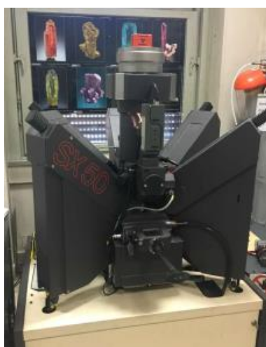
Figure 4.3 Electron microprobe CAMECA SX50
