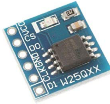
Figure 28 - Example of a 8MByte Dataflash Chip
