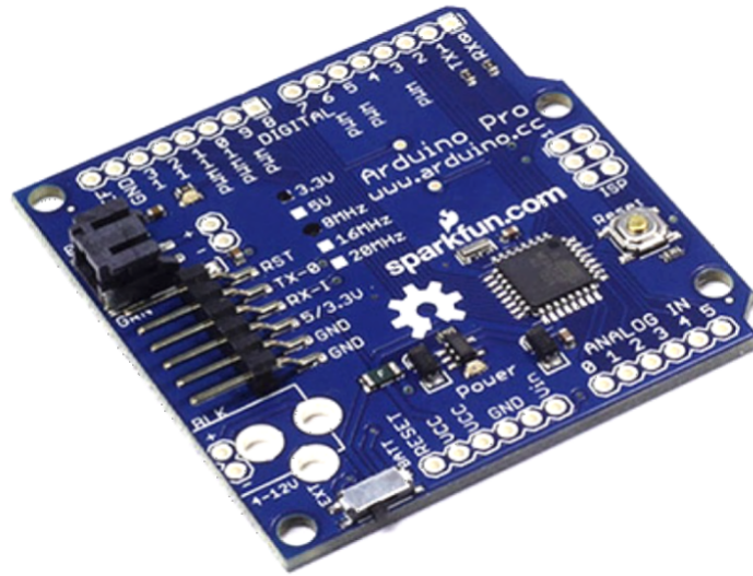
Figure 24 - Arduino Pro Board. Source: Arduino ( https://arduino.cc )
