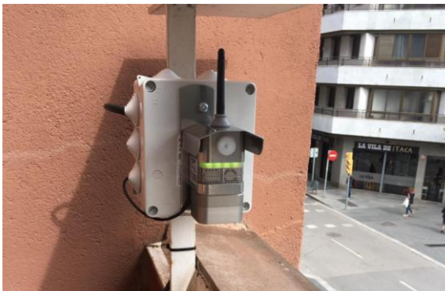
Image 14: AIRLY sensor in operation the balcony of the main building of the City of Sant Adrià de Besòs.
