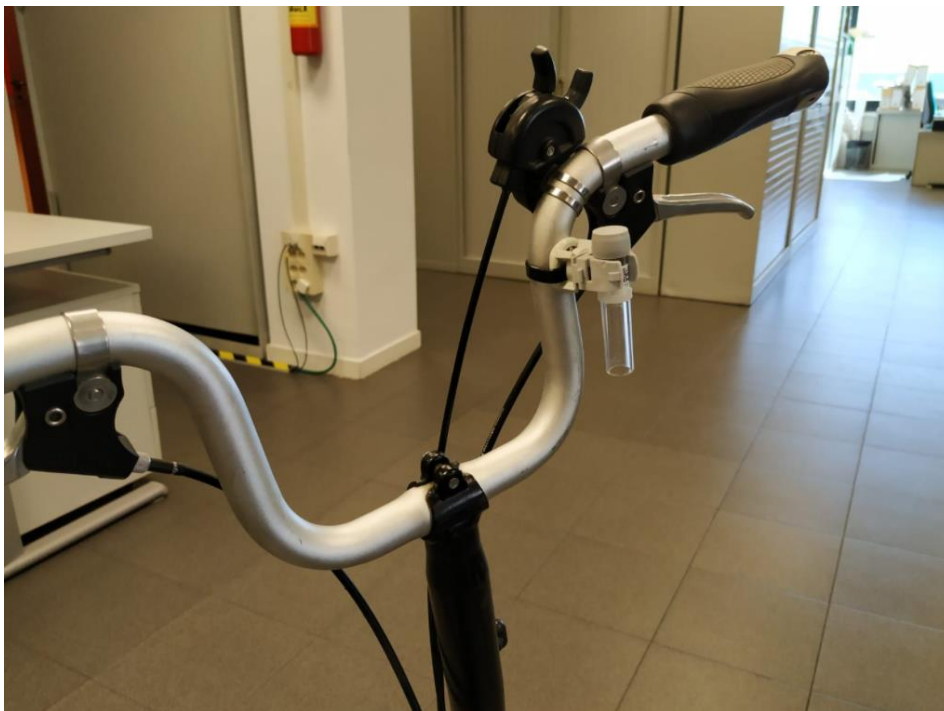
Image 12: Hooking system of the passive dosimeters on the bicycle of one of the volunteers.
