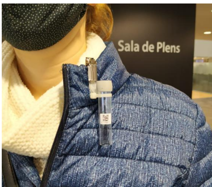
Image 10: Hooking system of the passive dosimeters on the clothing of one of the volunteers.
