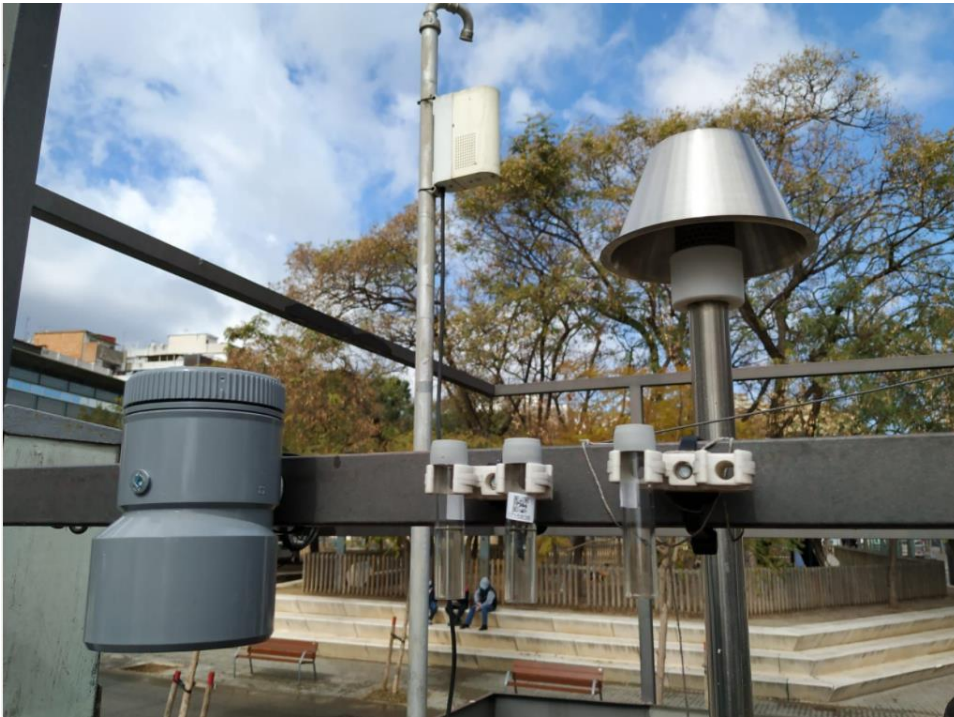
Image 11: Installation of the passive dosimeters in one of the automatic stations.
