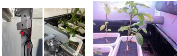
Figure 3. Camera placement for experiment; (a) Raspberry pi (RPI Zero W, Raspberry foundation) with camera installed on the side of the cultivation area, (b) Camera device (RPI 3B+, Raspberry foundation) for photographing single plant, (c) Snapshot of seedling of tea tree.
