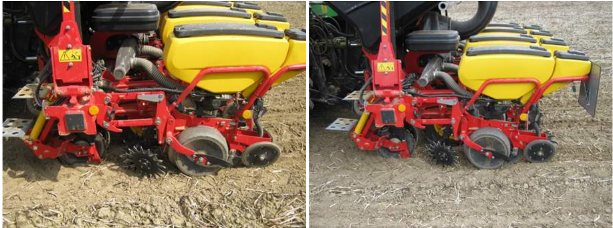
Figure 2. Variants without fixed row cleaner with standard closing wheels (left) and standard + structured closing wheels (right)
