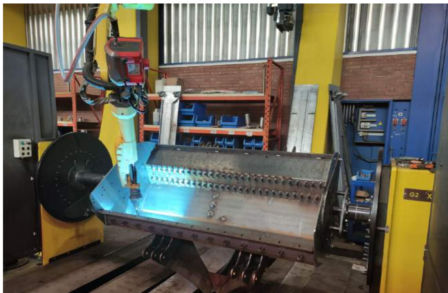
Figure 5. Machine welded with robot programmed offline.
