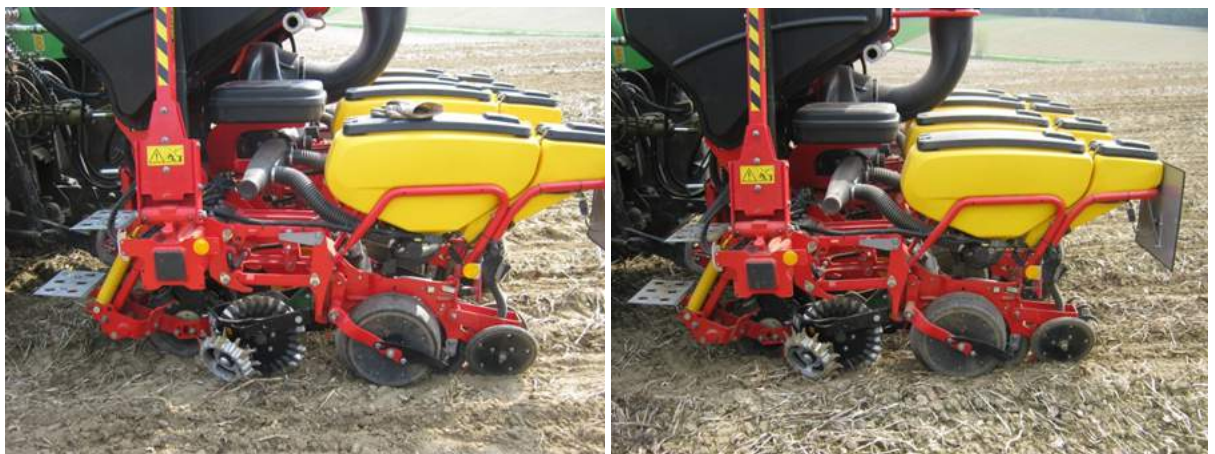
Figure 4. Variants without waved coulter plus floating row cleaners with standard closing wheels (left) and standard + structured closing wheels (right)
