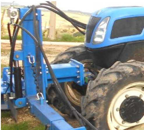
Figure 4 Implement headstock mounted at the front of the tractor
