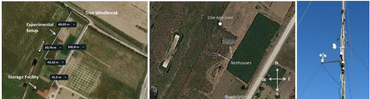
Figure 1. The experimental field; Field dimensions (left, Zoom Earth), magnified image (middle, Google Maps), anemometer and wind vane at 4m height
