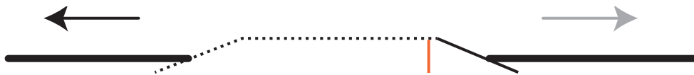
Figure 3: First part of further iteration of the concept design, Nov 2019: a moving structure with a grated top that collects fine particles by moving under a substrate. Source: authors' internal document.
