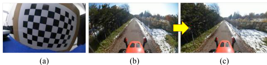
Figure 2. a) 9x6 grid chessboard, b) input image with camera distortion, c) resulting image without camera distortion
