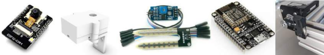
Figure 3. (a) ESP32-CAM, (b) Camera casing design, (c) Soil humidity sensor, (d) NodeMCU, (e) Limit switch.
