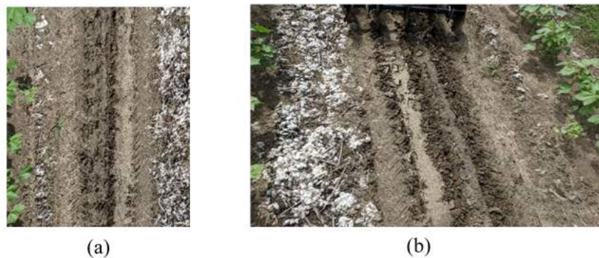
Figure 11. Weed control field trials results for (a) V-shaped weeder and (b) Harrow disk weeder.
