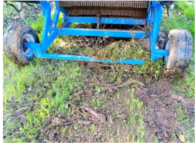
Figure 18. Insufficient clearance to the soil of the chassis
