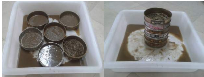
Figure 1. The sieves used for determining the particle size distribution of manure sample
