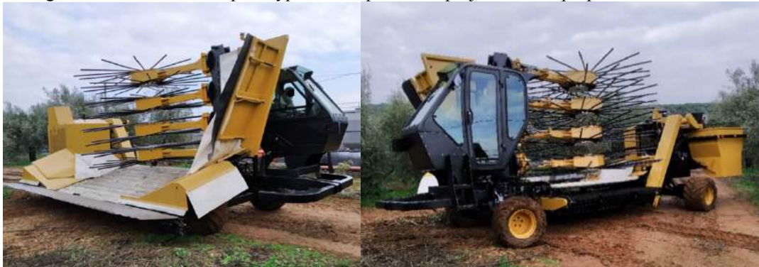
Figure 2. Olive harvester prototype developed in CPP Innolivar based on lateral canopy shaker.
