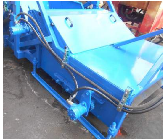
Figure 10. Hydraulic motors to drive transversal rotor and conveyor elevator
