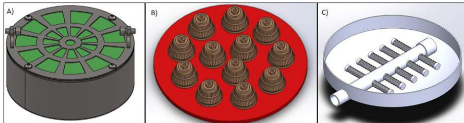
Figure 1. Different underdrain designs: porous media (A), inserted domes (B) and wand (C).
