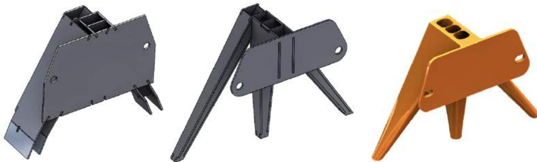
Figure 2. The 3D models (from L to R) of the original stainless-steel design, the improved stainless-steel design, and the ABS 3D printed design with acetone smoothing.
