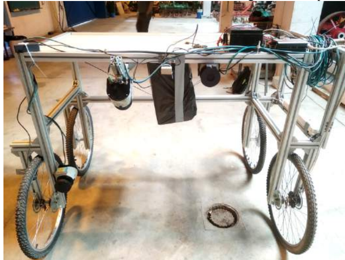
Figure 1. Structure implemented with aluminium profiles (45x45) and wheels.
