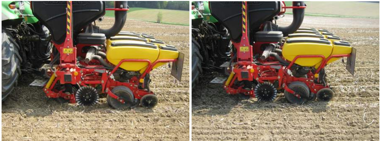
Figure 3. Variants without waved coulter with standard closing wheels (left) and standard + structured closing wheels (right)
