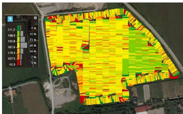
Figure 2. Map of the distributed dose (on the left in kg ha -1 ) from the C2 operator (MyJohnDeere). It's immediately clear the followed path and the practical advantages of the use of this technology.
