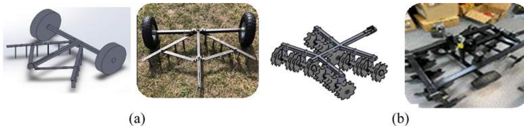
Figure 4. Two weeder designs tested for this work: (a) Weeder with V-shaped and (b) Weeder with adjustable harrow disk.
