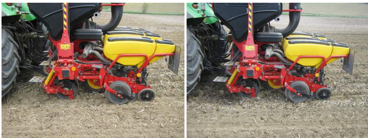
Figure 1. Variants without leading planter attachments with standard closing wheels (left) and standard + structured closing wheels (right)
