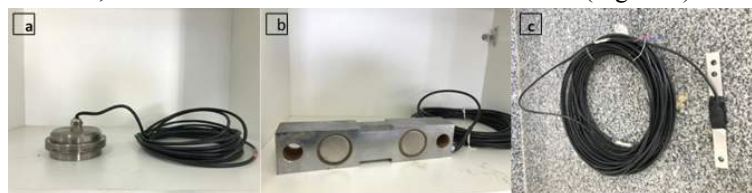
Figure 2. Types of measuring cells in the pilot silo. Pressure cell (a), shear beam load cell (b), tension load cell (c).
