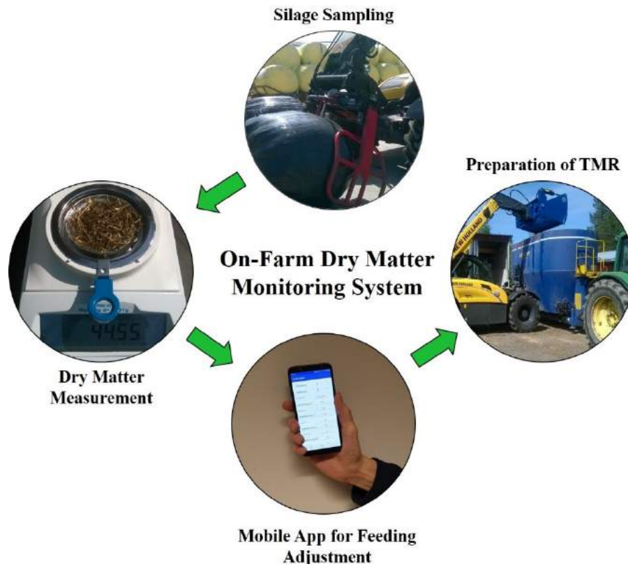
Figure 1. In the study, a system for regular monitoring of silage dry matter was developed and piloted at farms. It consisted of silage sampler attached to a bale gripper, on-farm dry matter measurement by a moisture analyser and a mobile application for TMR feeding adjustment.
