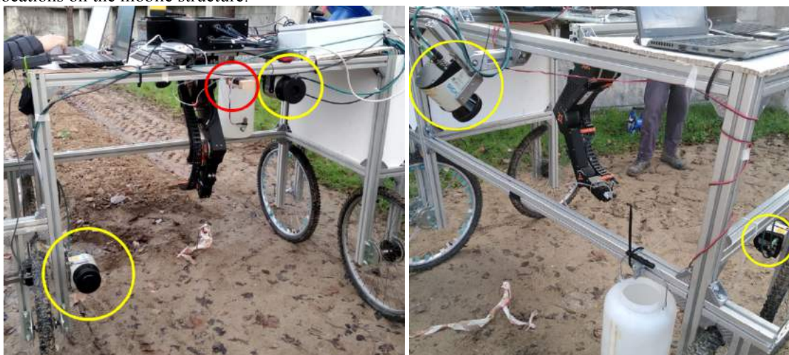
Figure 2. Frontal view (right) and rear of the platform (left), the yellow circles show the 3 lidar sensors and the red circle indicates the multispectral camera.
