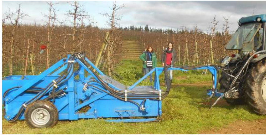
Figure 7. Lift and storage unit semi-mounted in the tractor
