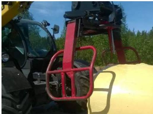
Figure 2. Silage sampling with the designed sampler. Figure 3. The sampling tube is emptied with a push-out rod.
