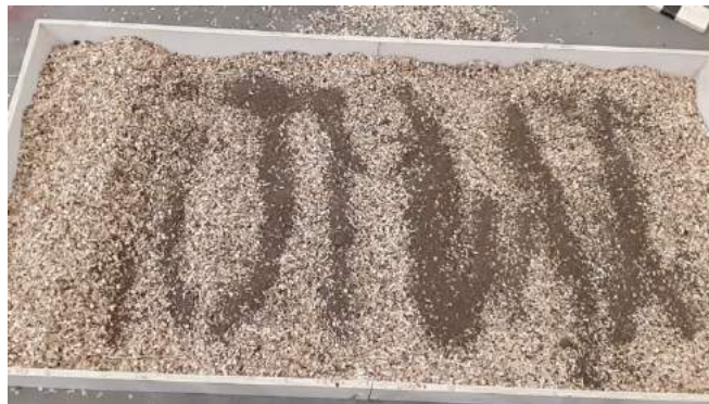
Figure 4: Wooden box filled with beech clippings and dry manure spread over the top
