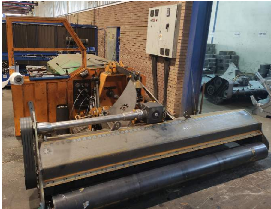
Figure 9. Manufactured machine undergoes no-load test.
