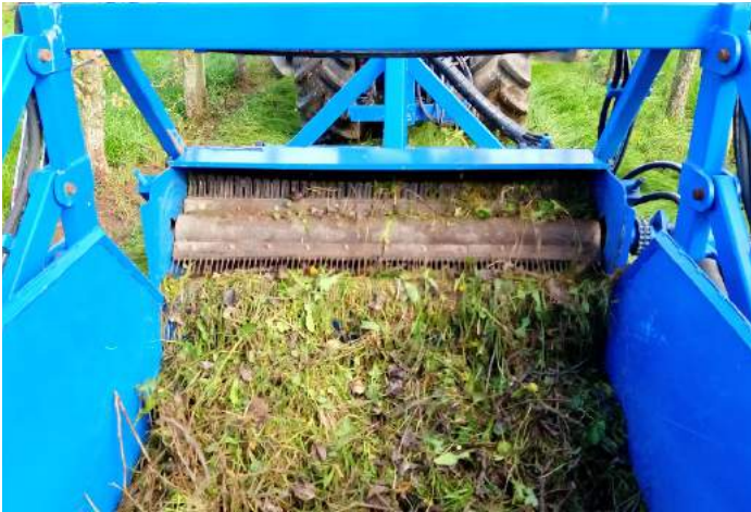
Figure 9. Rear view of conveyor elevator and storage box
