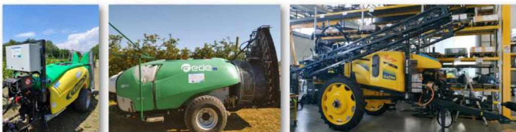
Figure 7. The three OPTIMA smart sprayers (for vineyards, apple orchards and open field carrots respectively)
