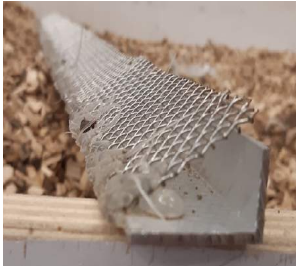
Figure 5: Detailed view of the first prototype, used to be moved manually under the beech clippings
