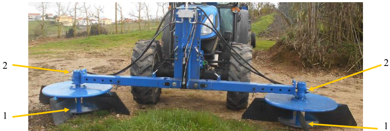
Legend: 1 – disc skid; 2 - hydraulic motors
