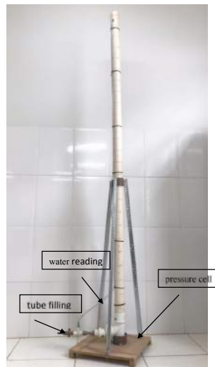
Figure 3. Tube to measure pressure - pressure cell calibration system.
