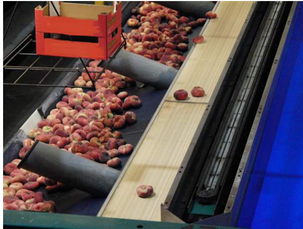
Figure 6: Transfer point: Fourth conveyor belt (to the packing tables) - Packing table
