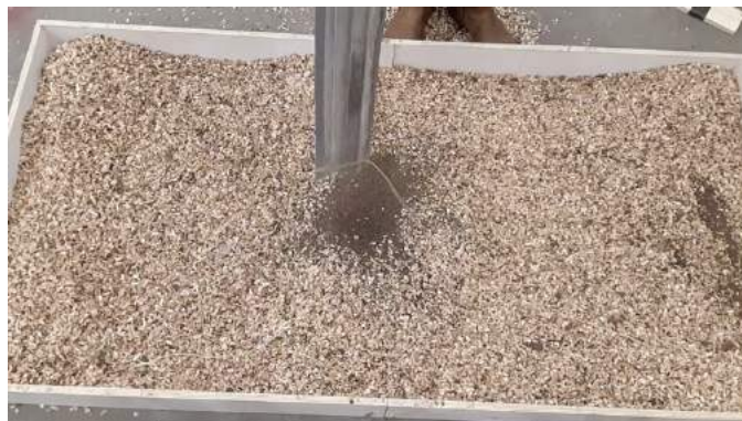
Figure 6: Prototype is emptied after being moved manually back and forth two times under the beech clippings
