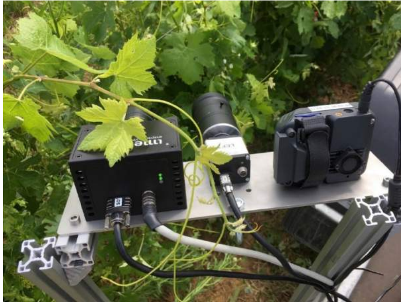
Figure 1. An example of the setup in the field and all three cameras imaging downy mildew
