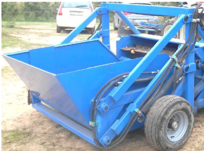
Figure 11. Temporary storage box mounted on pantograph arms
