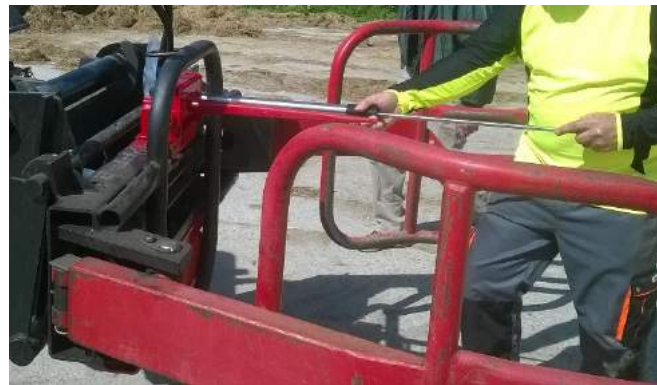
Figure 2. Silage sampling with the designed sampler. Figure 3. The sampling tube is emptied with a push-out rod.
