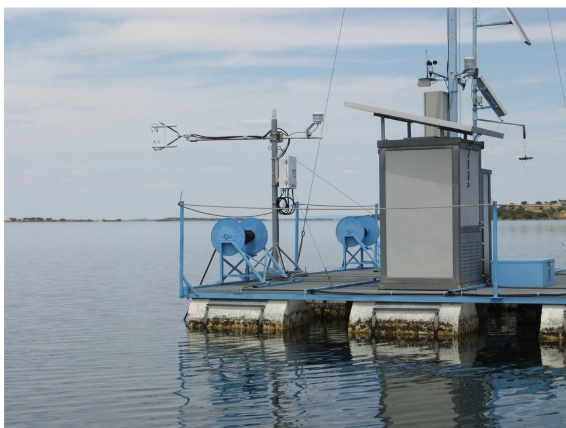
EC system (IRGASON; Campbell Scientific) installed on a floating platform at Alqueva reservoir, within the framework of the ALEX project ( www.alex2014.cge.uevora.pt )
