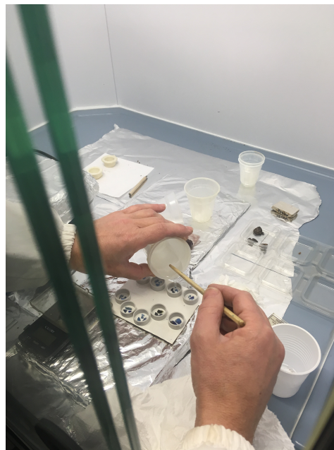
(b) Pouring the epoxy resin inside the mounted samples.
