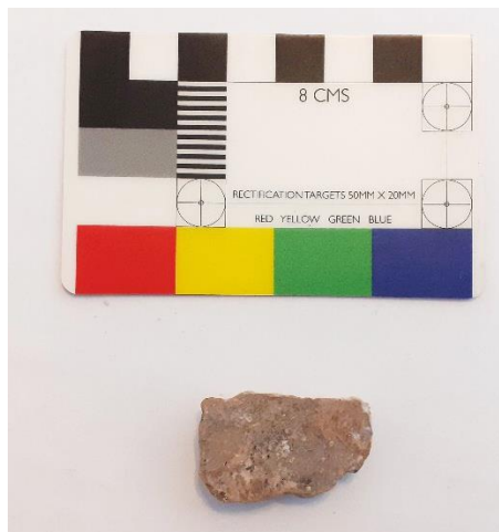
Figure 38 Sample 24 also appeared purple, but produced only large amounts of fluorescence with the BRAVO and only the spectra of calcite with the i-Raman.
