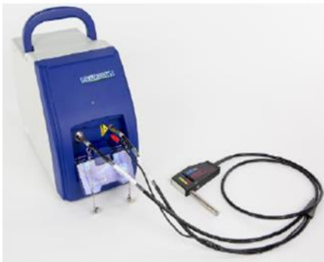
Figure 11 Left: i-Raman EX spectrometer. Photo © Metrohm SG, www.metrohm.com . Right: i-Raman set up, using a microscope stage for positioning.
