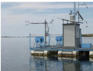
EC system (IRGASON; Campbell Scientific) installed on a floating platform at Alqueva reservoir, within the framework of the ALEX project (www.alex2014.cge.uevora.pt)
