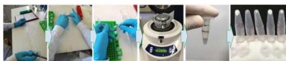
Fig. 3: Images showing several steps of the gDNA extraction procedure, going from removal of biological particles from the melinex tape till DNA precipitation.
