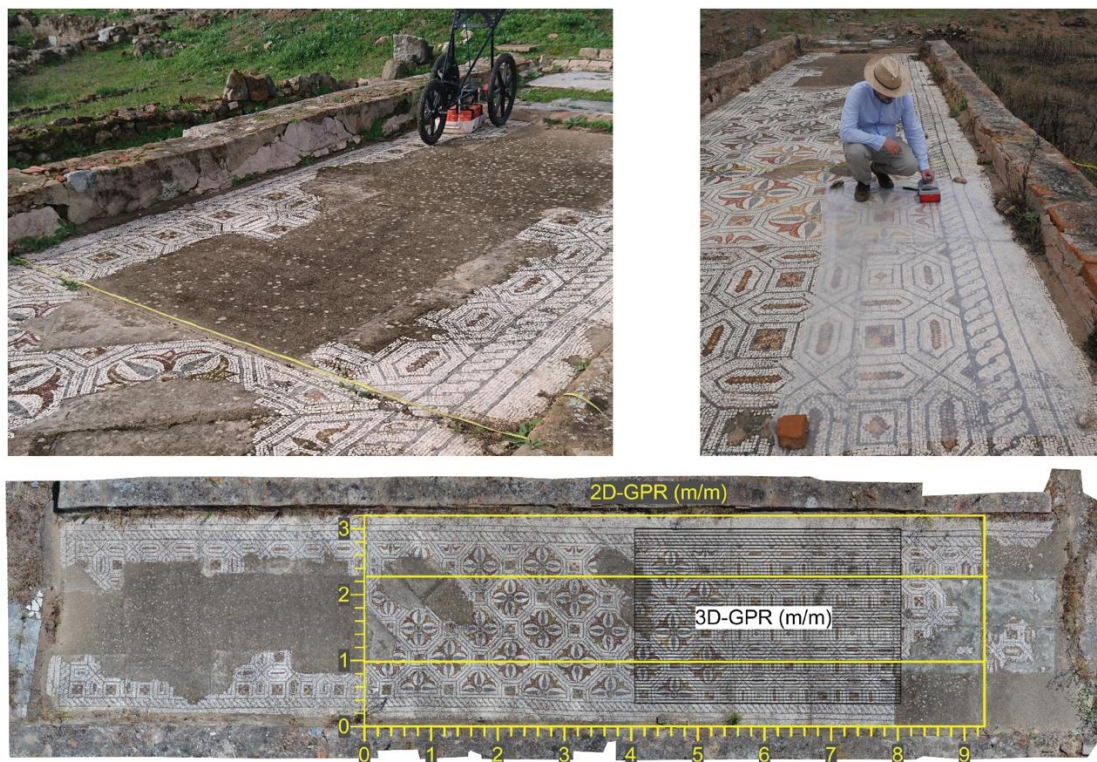
Figure 7. The upper left image shows the 400 MHz antenna, which was used in this study to generally inspect below the mosaic. In the upper right image shows the 1600 MHz antenna, which was used to conduct a detailed 3D inspection of the mosaic. The lower image corresponds to the orthomosaic of the corridor where the inspected rectangles were placed; in yellow, the area of the 2D ground penetrating radar (GPR) profiles; and in black, the 3D-GPR area with parallel profiles spaced 0.05 m apart.
