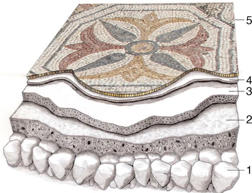
Figure 2. Stratigraphy of a Roman mosaic floor according to Vitruvius's description. The scheme is adapted from the Getty Conservation Institute and the Israel Antiquities Authorities and shows a fragment of the studied mosaic. 1. Statumen —First preparatory layer of large stones; 2. Rudus —mortar layer of gravel to level the floor; 3. Nucleus —impermeable mortar layer of powdered pottery and lime to protect the mosaic surface from the soil water (humidity); 4. Bedding —thin mortar layer, rich in lime, applied fresh in small regular portions where the mosaic designs were marked, and the tesserae were inserted before the mortar dried; and 5. Tessellatum —surface of the mosaic composed of tesserae and mortar with the bedding composition filling the interstices between tesserae .
