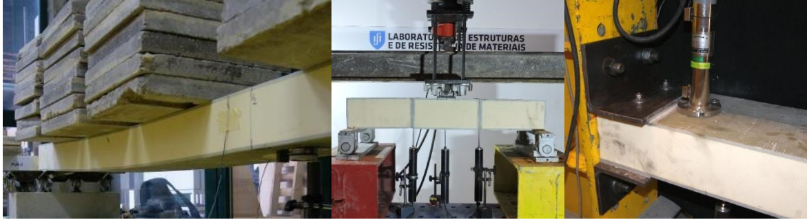
Figure 5. Research on GFRP sandwich panels for building floors rehabilitation (left to right): creep behaviour, panel-to-panel connections, panel-to-wall connections.
