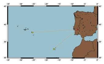
**Fig. 5.** Map of the planned VLF/LF radio broadcast system: three transmitters (represented by yellow squares) located at Azores (Portugal), Madeira (Portugal) and Ceuta (Spain), and the receiver (shown as a red star) installed at Évora (Portugal).
