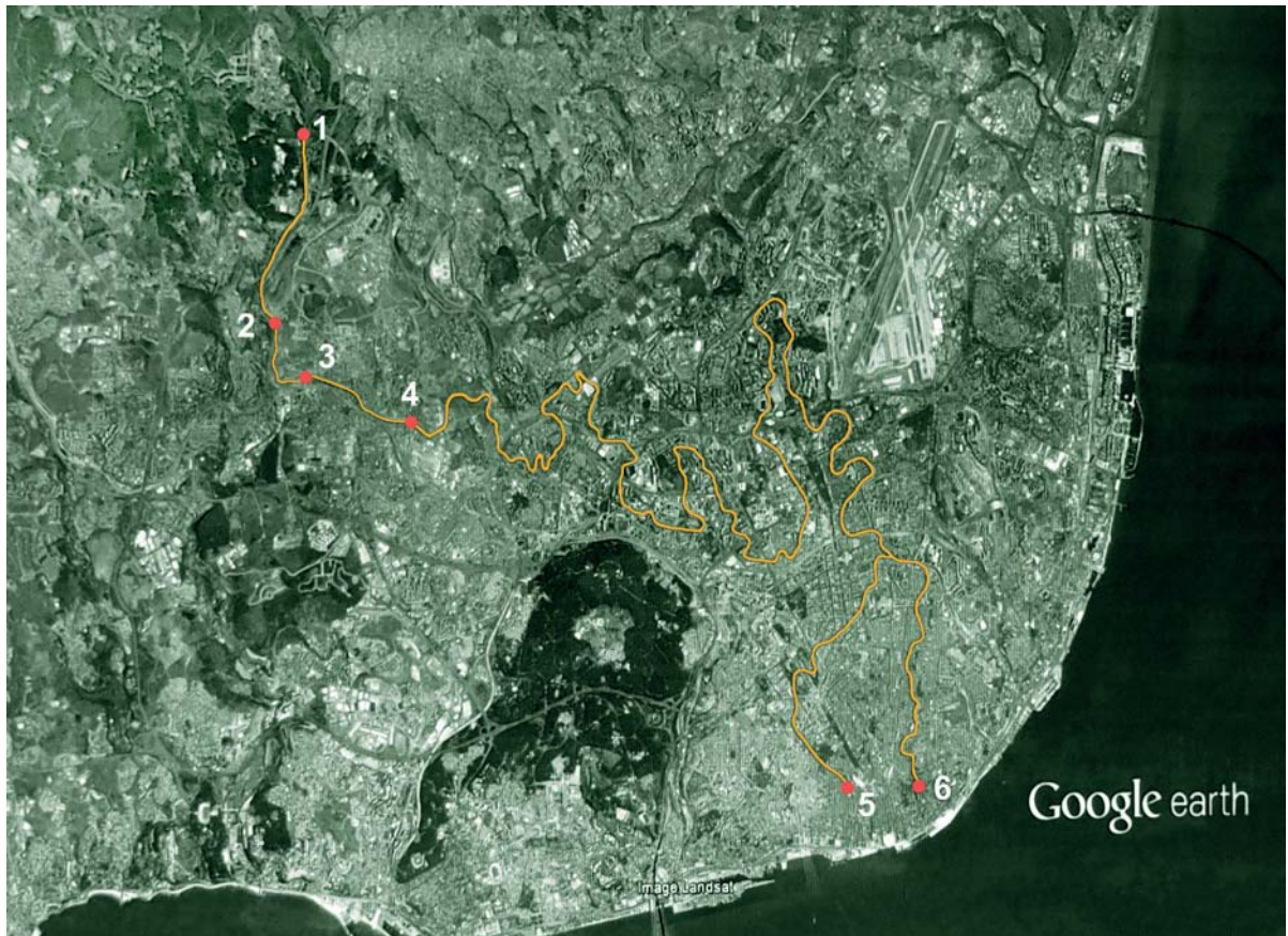
Fig. 10. Potential aqueduct route on 2016 Digital Globe / Google Earth satellite image: 1 Águas Livres springs and dam; 2-3 Sector with aqueduct archaeological remains; 4 Control test-point in Benfica old road; 5 São Roque site; 6 Santo André gate (after Nuno Sousa Neves).
