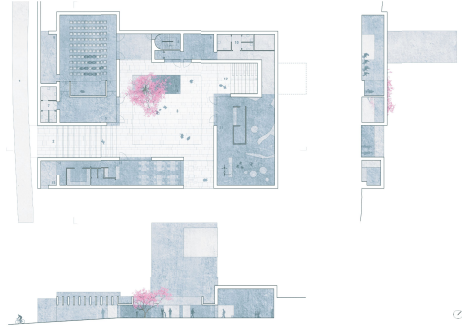
1 terrace / greenwood forest | 2 pre-existing industrial site | 3 stair path | 4 POCCI patio / courtyard | 5 interpretative center | 7 outdoor | 8 auditorium 9 panoramic platform | 10 main access | 11 water mirror | 12 perspective | 13 wall | 14 technical platform | 15 stairs panoramic platform | 16 kitchen | 17 technical base outside
