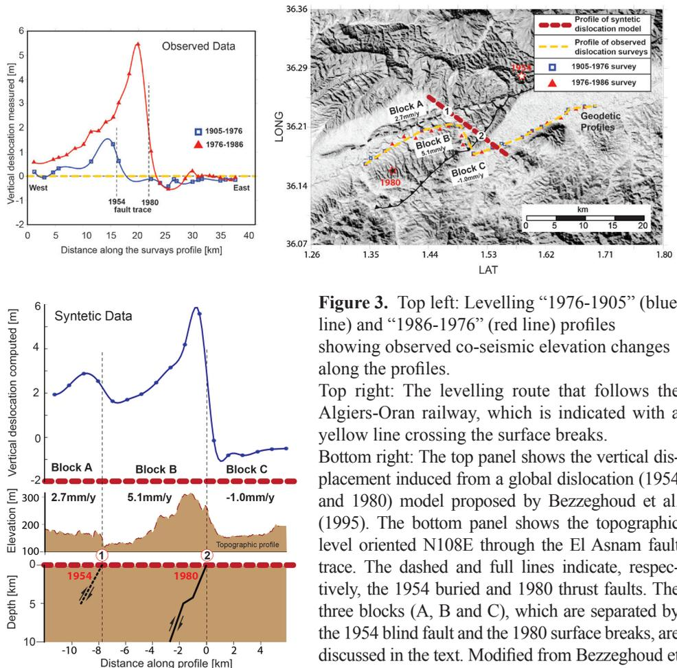
**Figure 3.** Top left: Levelling “1976-1905” (blue line) and “1986-1976” (red line) profiles showing observed co-seismic elevation changes along the profiles.
