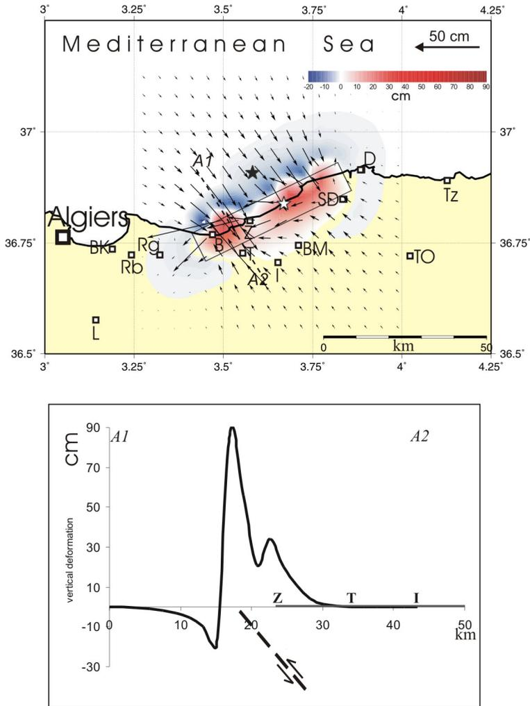
**Figure 7.** Predicted co-seismic displacement field model. Top: Vertical and horizontal co-seismic distribution map. Blue and red colors indicate, respectively, subsidence and uplift. Bottom: profile along A1-A2 from top of figure.
