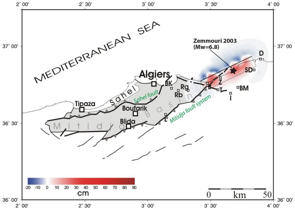
**Figure 8.** Predicted co-seismic vertical displacement map plotted together with the tectonic background of the epicentral area and the main shock epicenter represented by the open star.
