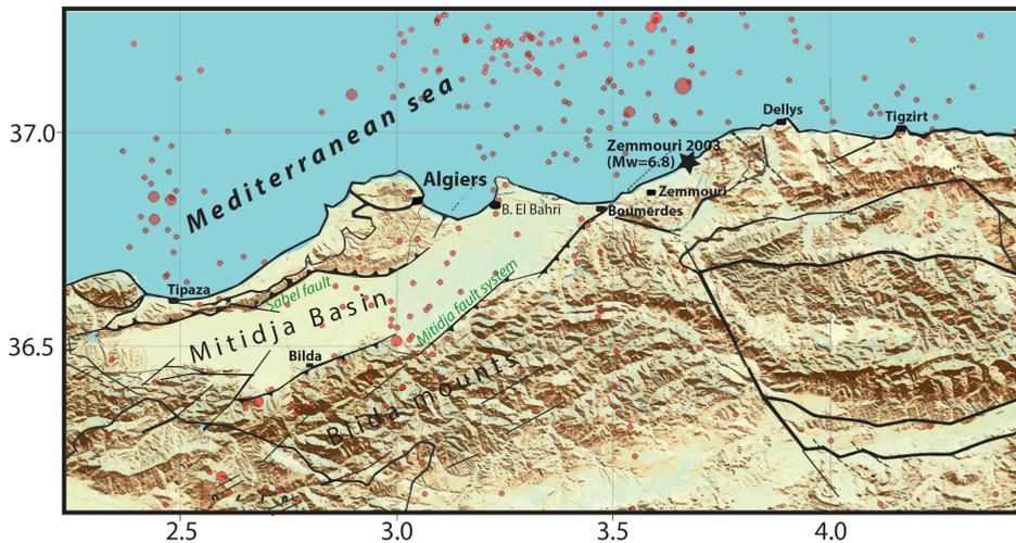
**Figure 4.** Tectonic and seismicity ( $M \geq 4.0$ , 1910-2016) map of the Mitidja basin (central Algeria). The tectonic framework is adapted from Ayadi et al. (2003) and the seismic data were taken from the ISC database.
