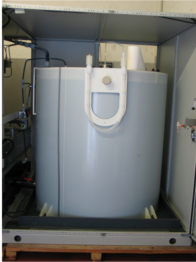
Figure 4.10: Photograph of the positive tank (catholyte tank) of the prototype VRFB system. Each tank holds approximately 1800 liters of electrolyte. The pipes with larger diameter (blue colour) transport the electrolyte through the piping system while the translucent pipes provide the inert gas used to act as a “blanket”.
