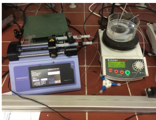
Figure 3.26: Flow chemistry setup used for our reactions.
