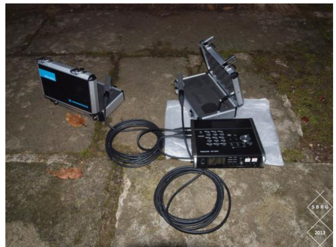
Figure 2. The set used for recording in the Abbey of San Salvatore: the recorder Tascam DR-680 and Sennheiser MKH 8020 microphones
