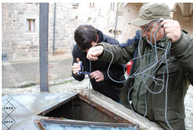
Figure 4. two microphones Hydrophones being placed in the well, despite a cable length of 12 meters, they did not resting on the bottom of the tank
