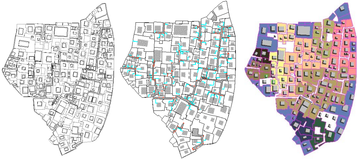
Figure 18. Plan of Zaouiat Lakhdar displaying the superimposition of drawing information (collected in situ with official data). The drawing shows discrepancies that were corrected.
