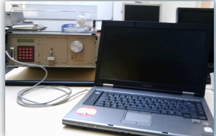
Meter of atmospheric Radon levels (in installation).
