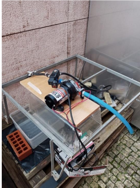
Figure 5. Photo of the setup of the pump used for performing the overspraying.
