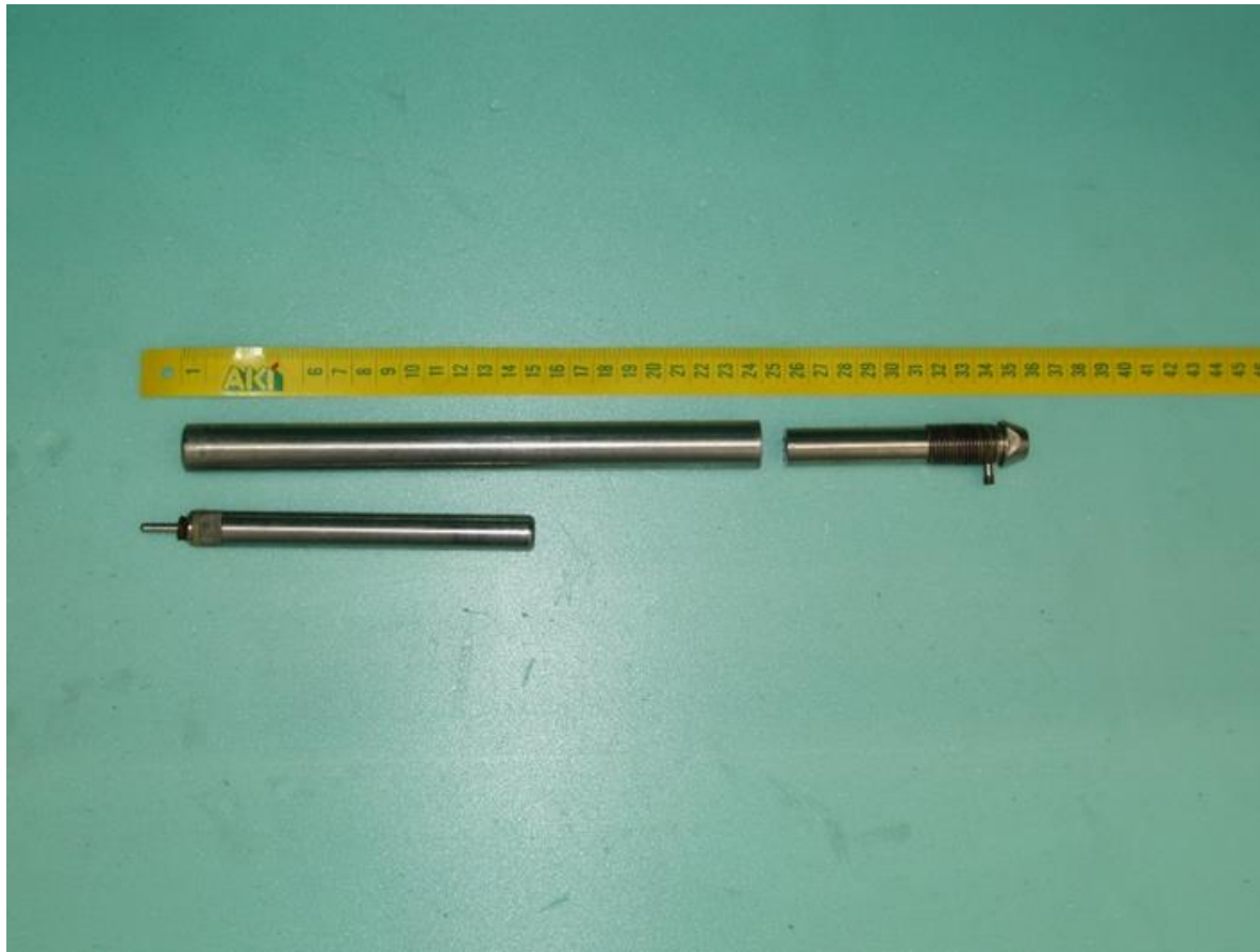
ANTARES Datalogger. SN-185 42 50 and protection casing
