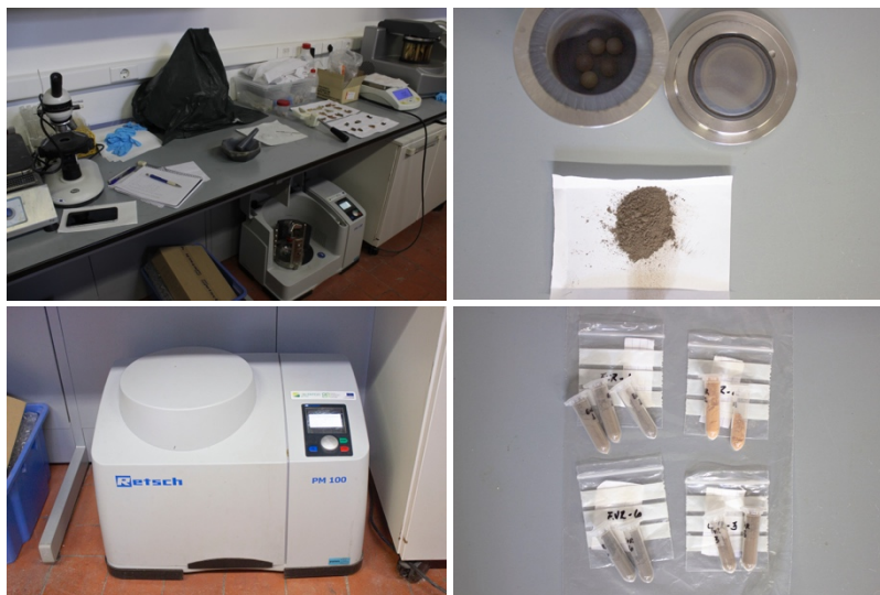
Figure 44. Use of an agate mortar for the first hand-crushing (upper left). 45. A full ground using an automatic mill machine (lower left). 46. Solid ceramic balls inside a drum are involved in the ground process (upper right). 47. Fine powder specimens were preserved in small plastic containers and labelled (lower right).
