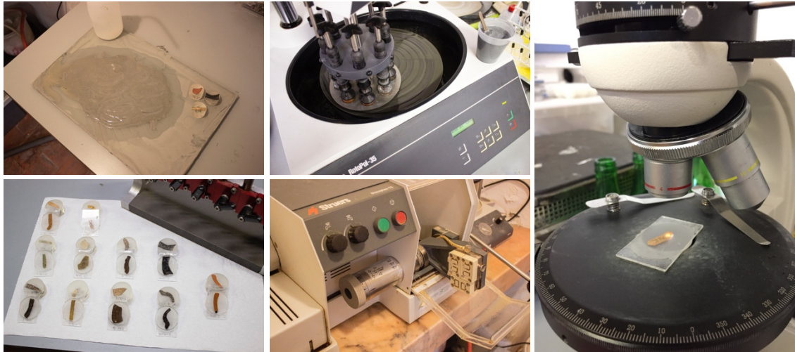
Figure 58. Hand polishing of polish blocks using a SiC grit, water and a flat, thick glass (upper left). 59. A semi-automatically polishing-lapping device was used in the process (middle up). 60. Glass slides attached to the resin blocks ready for polishing (lower left). 61. Mechanical polishing of glass slides by means of a diamond-covered rotating wheel (middle down). 62. Leveling of the glass slides were checked out through the interference colour pattern using and microscope (right).
