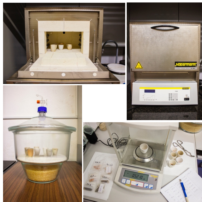
Figure 50. Ceramic crucibles inside the furnace for the calcination (upper left). 51. A furnace where the calcination of fine powder specimens was carried out (upper right). 52. Desiccator with silica gel and crucibles getting cold inside in a dry environment. 53. Measuring the respective weights of crucibles and specimens (lower right).
