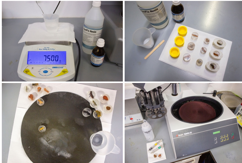
Figures 54. A particular resin and hardener mixed together for making the epoxy resin (upper left). 55. Epoxy resin was poured into a small cups with the chips inside (upper right). 56. Process of hand-polishing for removing resin remnants (lower left). 57. A semi-automatically polishing-lapping machine with a coupled rotary platform for the finishing polishing onto a velvet-coated magnetic foil (lower right).
