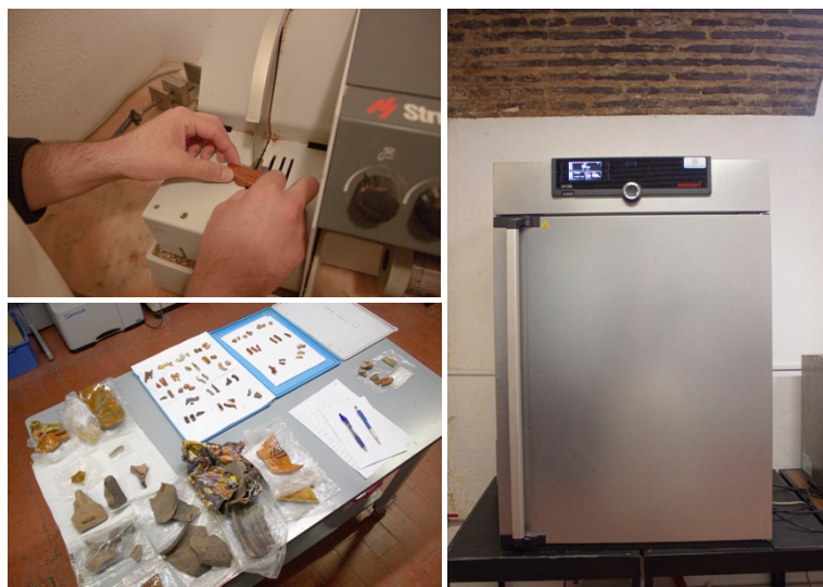
Figure 41. Process of cutting off the bulk samples (upper left). 42. Displaying of the sectioned ceramic pieces (lower left). 43. Drying chamber where were kept the chips after the sectioning procedure (right).
