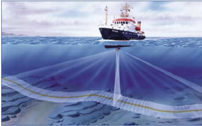
Fig. 5.1.1 Basic principle of a multi-beam echosounder.
