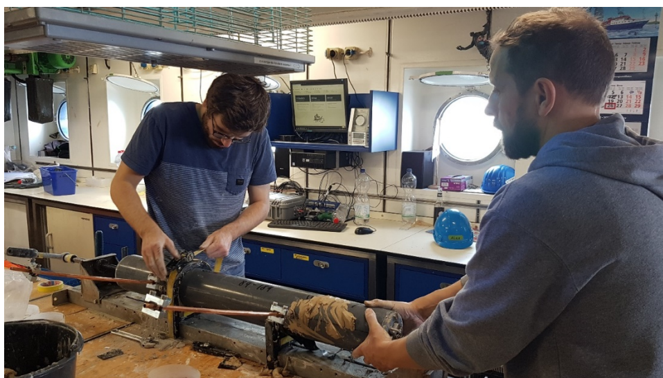
Fig. 5.6.8 Sediment sampling from core segments for noble gas analysis used during M162.
